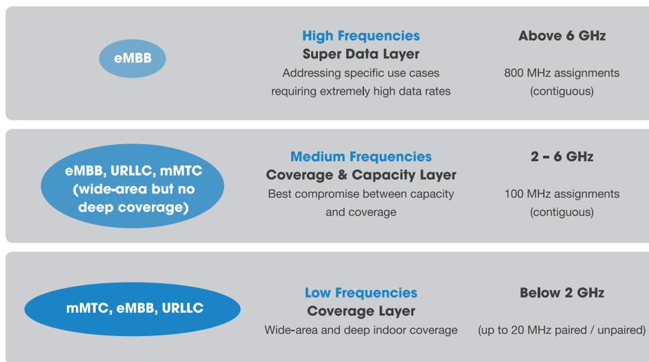
**Figure 2: 5G Spectrum Bands allocated to 5G use cases (Source Huawei)**
