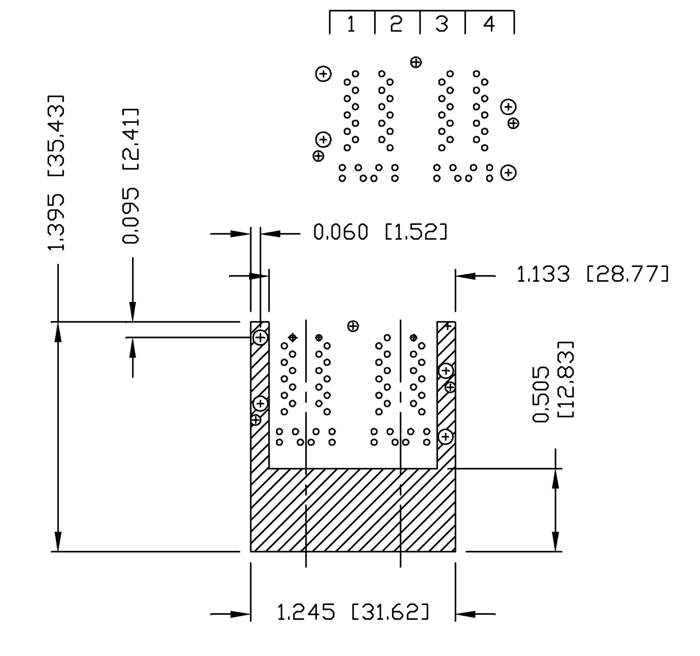
THE SHADED AREA ON THE CUSTOMER BOARD ARE RECOMMENDED TO BE CLEAR OFF ANY VIA HOLE OR COMPONENT PAD.
