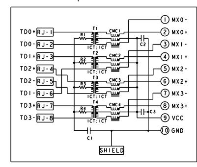
C1 = 1000pF, 2kV Capacitor C2 - C3 = 10nF, 50V Capacitors R1-R4 = 75 Ohms, 1/16 W, Resistors
