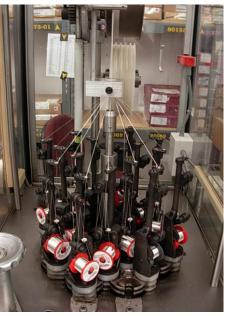
\*Excessive handling can deteriorate IL performance. No unnecessary re-spooling of cable prior to extrusion.
