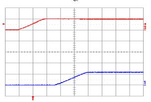
Fig. 1.2V.4: Turn-on transient for Vout = 1.2 V with application of Vin at full rated load current (resistive) and 100 μF external capacitance at Vin = 5 V. Top trace: Vin (5 V/div.); Bottom trace: output voltage (1 V/div.); Time scale: 2 ms/div.
