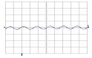
Fig. 2.0V.5: Output voltage ripple (20 mV/div.) at full rated load current into a resistive load with external capacitance  $100 \, \mu F$  ceramic +  $1 \, \mu F$  ceramic and Vin =  $5 \, V$  for Vout =  $2.0 \, V$ . Time scale:  $2 \, \mu s$ /div.
