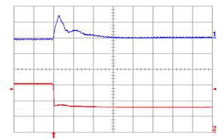
Fig. 1.2V.7: Output voltage response for Vout = 1.2 V to negative load current step change from 16 A to 8 A with slew rate of -5 A/μs at Vin = 5 V. Top trace: output voltage (100 mV/div.); Bottom trace: load current (5 A/div.). Co = 100 μF ceramic + 1 μF ceramic. Time scale: 20 μs/div.
