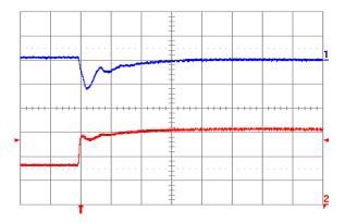
Fig. 0.7525V.6: Output voltage response for Vout = 0.7525 V to positive load current step change from 8 A to 16 A with slew rate of 5 A/μs at Vin = 5 V. Top trace: output voltage (100 mV/div.); Bottom trace: load current (5 A/div.). Co = 100 μF ceramic + 1 μF ceramic. Time scale: 20 μs/div.
