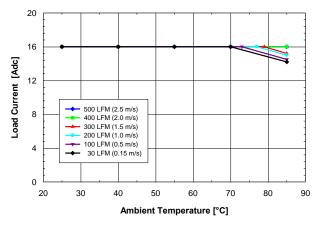
Fig. 1.5V.1: Available load current vs. ambient temperature and airflow rates for Vout = 1.5 V converter mounted vertically with Vin = 5 V, air flowing from pin 10 to pin 1, and maximum MOSFET temperature  $\leq$  120 °C.
