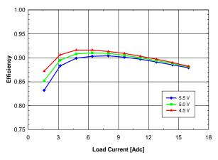
Fig. 1.5V.2: Efficiency vs. load current and input voltage for Vout = 1.5 V converter mounted vertically with air flowing from pin 10 to pin 1 at a rate of 200 LFM (1 m/s) and Ta = 25
