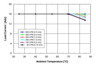
Fig. 3.3V.1: Available load current vs. ambient temperature and airflow rates for Vout = 3.3 V converter mounted vertically with Vin = 5 V, air flowing from pin 10 to pin 1, and maximum MOSFET temperature  $\leq 120 \text{ }^{\circ}\text{C}$ .
