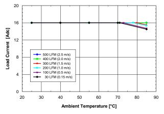
Fig. 1.2V.1: Available load current vs. ambient temperature and airflow rates for Vout = 1.2 V converter mounted vertically with Vin = 5 V, air flowing from pin 10 to pin 1, and maximum MOSFET temperature  $\leq$  120 °C.
