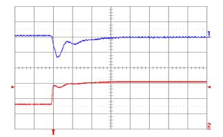
Fig. 1.0V.6: Output voltage response for Vout = 1.0 V to positive load current step change from 8 A to 16 A with slew rate of 5 A/μs at Vin = 5 V. Top trace: output voltage (100 mV/div.); Bottom trace: load current (5 A/div.). Co = 100 μF ceramic + 1 μF ceramic. Time scale: 20 μs/div.
