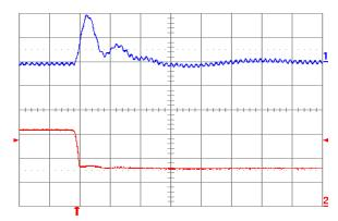
Fig. 2.5V.7: Output voltage response for Vout = 2.5 V to negative load current step change from 16 A to 8 A with slew rate of -5 A/μs at Vin = 5 V. Top trace: output voltage (100 mV/div.); Bottom trace: load current (5 A/div.). Co = 100 μF ceramic + 1 μF ceramic. Time scale: 20 μs/div.
