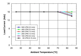
Fig. 1.8V.1: Available load current vs. ambient temperature and airflow rates for Vout = 1.8 V converter mounted vertically with Vin = 5 V, air flowing from pin 10 to pin 1, and maximum MOSFET temperature  $\leq$  120 °C.
