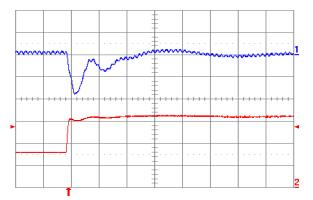
Fig. 2.5V.6: Output voltage response for Vout = 2.5 V to positive load current step change from 8 A to 16 A with slew rate of 5 A/μs at Vin = 5 V. Top trace: output voltage (100 mV/div.); Bottom trace: load current (5 A/div.). Co = 100 μF ceramic + 1 μF ceramic. Time scale: 20 μs/div.
