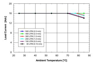
Fig. 2.0V.1: Available load current vs. ambient temperature and airflow rates for Vout = 2.0 V converter mounted vertically with Vin = 5 V, air flowing from pin 10 to pin 1, and maximum MOSFET temperature  $\leq 120 \text{ }^{\circ}\text{C}$ .
