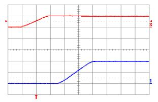
Fig. 2.0V.4: Turn-on transient for Vout = 2.0 V with application of Vin at full rated load current (resistive) and 100 μF external capacitance at Vin = 5 V. Top trace: Vin (5 V/div.); Bottom trace: output voltage (1 V/div.); Time scale: 2 ms/div.
