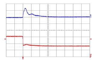
Fig. 0.7525V.7: Output voltage response for Vout = 0.7525 V to negative load current step change from 16 A to 8 A with slew rate of -5 A/μs at Vin = 5 V. Top trace: output voltage (100 mV/div.); Bottom trace: load current (5 A/div.). Co = 100 μF ceramic + 1 μF ceramic. Time scale: 20 μs/div.
