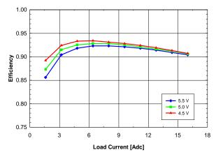
Fig. 2.0V.2: Efficiency vs. load current and input voltage for Vout = 2.0 V converter mounted vertically with air flowing from pin 10 to pin 1 at a rate of 200 LFM (1 m/s) and Ta = 25
