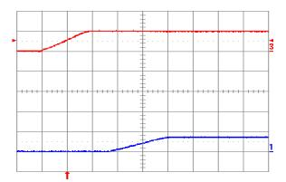
Fig. 0.7525V.4: Turn-on transient for Vout = 0.7525V with application of Vin at full rated load current (resistive) and 100 μF external capacitance at Vin = 5 V. Top trace: Vin (5 V/div.); Bottom trace: output voltage (1 V/div.); Time scale: 2 ms/div.
