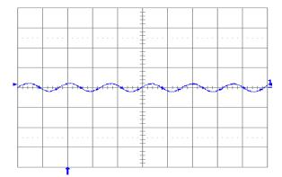
Fig. 1.8V.5: Output voltage ripple (20 mV/div.) at full rated load current into a resistive load with external capacitance 100 μF ceramic + 1 μF ceramic and Vin = 5 V for Vout = 1.8 V. Time scale: 2 μs/div.
