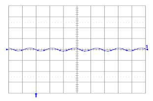
Fig. 1.2V.5: Output voltage ripple (20 mV/div.) at full rated load current into a resistive load with external capacitance  $100 \, \mu F$  ceramic +  $1 \, \mu F$  ceramic and Vin =  $5 \, V$  for Vout =  $1.2 \, V$ . Time scale:  $2 \, \mu s$ /div.
