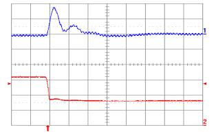
Fig. 2.0V.7: Output voltage response for Vout = 2.0 V to negative load current step change from 16 A to 8 A with slew rate of -5 A/μs at Vin = 5 V. Top trace: output voltage (100 mV/div.); Bottom trace: load current (5 A/div.). Co = 100 μF ceramic + 1 μF ceramic. Time scale: 20 μs/div.
