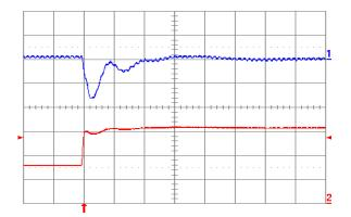
Fig. 1.8V.6: Output voltage response for Vout = 1.8 V to positive load current step change from 8 A to 16 A with slew rate of 5 A/μs at Vin = 5 V. Top trace: output voltage (100 mV/div.); Bottom trace: load current (5 A/div.). Co = 100 μF ceramic + 1 μF ceramic. Time scale: 20 μs/div.
