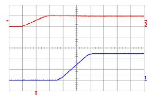
Fig. 2.5V.4: Turn-on transient for Vout = 2.5 V with application of Vin at full rated load current (resistive) and 100 μF external capacitance at Vin = 5 V. Top trace: Vin (5 V/div.); Bottom trace: output voltage (1 V/div.); Time scale: 2 ms/div.
