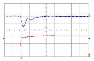
Fig. 1.5V.6: Output voltage response for Vout = 1.5 V to positive load current step change from 8 A to 16 A with slew rate of 5 A/μs at Vin = 5 V. Top trace: output voltage (100 mV/div.); Bottom trace: load current (5 A/div.). Co = 100 μF ceramic + 1 μF ceramic. Time scale: 20 μs/div.
