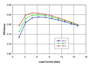
Fig. 0.7525V.2: Efficiency vs. load current and input voltage for Vout = 0.7525 V converter mounted vertically with air flowing from pin 10 to pin 1 at a rate of 200 LFM (1 m/s) and Ta = 25 °C.
