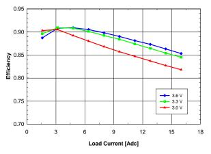
Fig. 1.2V.3: Efficiency vs. load current and input voltage for Vout = 1.2 V converter mounted vertically with air flowing from pin 10 to pin 1 at a rate of 200 LFM (1 m/s) and Ta = 25
