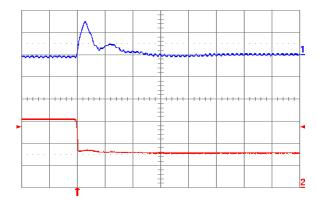
Fig. 1.5V.7: Output voltage response for Vout = 1.5 V to negative load current step change from 16 A to 8 A with slew rate of -5 A/μs at Vin = 5 V. Top trace: output voltage (100 mV/div.); Bottom trace: load current (5 A/div.). Co = 100 μF ceramic + 1 μF ceramic. Time scale: 20 μs/div.
