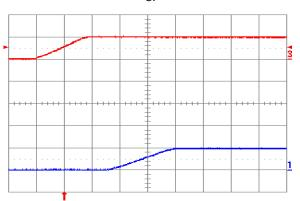
Fig. 1.0V.4: Turn-on transient for Vout = 1.0 V with application of Vin at full rated load current (resistive) and 100 μF external capacitance at Vin = 5 V. Top trace: Vin (5 V/div.); Bottom trace: output voltage (0.5 V/div.); Time scale: 2 ms/div.
