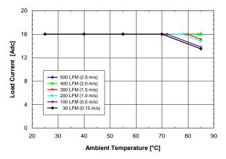
Fig. 2.5V.1: Available load current vs. ambient temperature and airflow rates for Vout = 2.5 V converter mounted vertically with Vin = 5 V, air flowing from pin 10 to pin 1, and maximum MOSFET temperature  $\leq 120 \text{ °C}$ .
