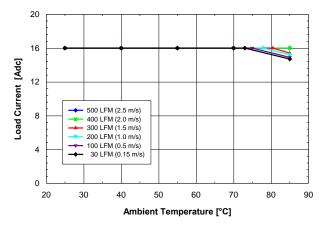
Fig. 1.0V.1: Available load current vs. ambient temperature and airflow rates for Vout = 1.0 V converter mounted vertically with Vin = 5 V, air flowing from pin 10 to pin 1, and maximum MOSFET temperature  $\leq 120 \text{ }^{\circ}\text{C}$ .
