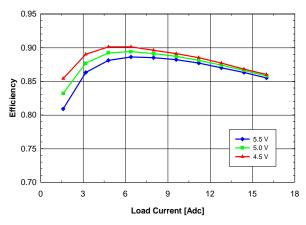
Fig. 1.2V.2: Efficiency vs. load current and input voltage for Vout = 1.2 V converter mounted vertically with air flowing from pin 10 to pin 1 at a rate of 200 LFM (1 m/s) and Ta = 25
