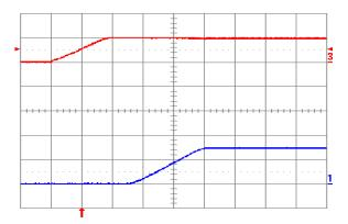
Fig. 1.5V.4: Turn-on transient for Vout = 1.5 V with application of Vin at full rated load current (resistive) and 100 μF external capacitance at Vin = 5 V. Top trace: Vin (5 V/div.); Bottom trace: output voltage (1 V/div.); Time scale: 2 ms/div.
