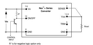
Fig. C: Circuit configuration for ON/OFF function.
