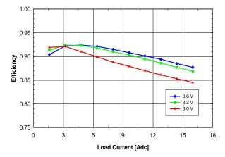
Fig. 1.5V.3: Efficiency vs. load current and input voltage for Vout = 1.5 V converter mounted vertically with air flowing from pin 10 to pin 1 at a rate of 200 LFM (1 m/s) and Ta = 25
