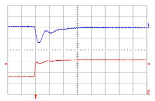
Fig. 1.2V.6: Output voltage response for Vout = 1.2 V to positive load current step change from 8 A to 16 A with slew rate of 5 A/μs at Vin = 5 V. Top trace: output voltage (100 mV/div.); Bottom trace: load current (5 A/div.). Co = 100 μF ceramic + 1 μF ceramic. Time scale: 20 μs/div.
