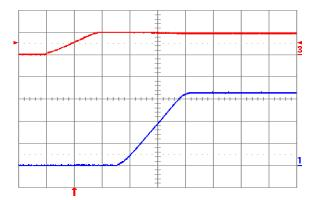
Fig. 3.3V.4: Turn-on transient for Vout = 3.3 V with application of Vin at full rated load current (resistive) and 100 μF external capacitance at Vin = 5 V. Top trace: Vin (5 V/div.); Bottom trace: output voltage (1 V/div.); Time scale: 2 ms/div.
