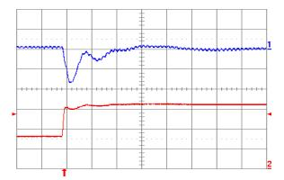
Fig. 2.0V.6: Output voltage response for Vout = 2.0 V to positive load current step change from 8 A to 16 A with slew rate of 5 A/μs at Vin = 5 V. Top trace: output voltage (100 mV/div.); Bottom trace: load current (5 A/div.). Co = 100 μF ceramic + 1 μF ceramic. Time scale: 20 μs/div.
