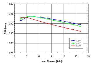
Fig. 1.8V.3: Efficiency vs. load current and input voltage for Vout = 1.8 V converter mounted vertically with air flowing from pin 10 to pin 1 at a rate of 200 LFM (1 m/s) and Ta = 25 °C.
