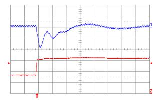
Fig. 3.3V.6: Output voltage response for Vout = 3.3 V to positive load current step change from 8 A to 16 A with slew rate of 5 A/μs at Vin = 5 V. Top trace: output voltage (100 mV/div.); Bottom trace: load current (5 A/div.). Co = 100 μF ceramic + 1 μF ceramic. Time scale: 20 μs/div.
