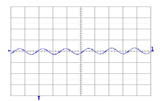
Fig. 2.5V.5: Output voltage ripple (20 mV/div.) at full rated load current into a resistive load with external capacitance  $100 \,\mu\text{F}$  ceramic +  $1 \,\mu\text{F}$  ceramic and Vin =  $5 \,\text{V}$  for Vout =  $2.5 \,$  V. Time scale:  $2 \,\mu\text{s}/\text{div}$ .
