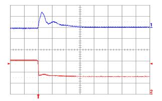
Fig. 1.0V.7: Output voltage response for Vout = 1.0 V to negative load current step change from 16 A to 8 A with slew rate of -5 A/μs at Vin = 5 V. Top trace: output voltage (100 mV/div.); Bottom trace: load current (5 A/div.). Co = 100 μF ceramic + 1 μF ceramic. Time scale: 20 μs/div.
