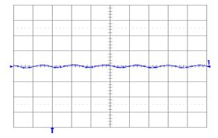
Fig. 0.7525V.5: Output voltage ripple (20 mV/div.) at full rated load current into a resistive load with external capacitance 100 μF ceramic + 1 μF ceramic and Vin = 5 V for Vout = 0.7525 V. Time scale: 2 μs/div.
