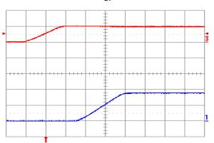
Fig. 1.8V.4: Turn-on transient for Vout = 1.8 V with application of Vin at full rated load current (resistive) and 100 μF external capacitance at Vin = 5 V. Top trace: Vin (5 V/div.); Bottom trace: output voltage (1 V/div.); Time scale: 2 ms/div.
