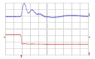
Fig. 3.3V.7: Output voltage response for Vout = 3.3 V to negative load current step change from 16 A to 8 A with slew rate of -5 A/μs at Vin = 5 V. Top trace: output voltage (100 mV/div.); Bottom trace: load current (5 A/div.). Co = 100 μF ceramic + 1 μF cera-mic. Time scale: 20 μs/div.
