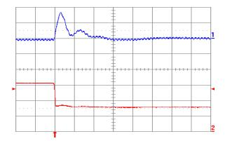
Fig. 1.8V.7: Output voltage response for Vout = 1.8 V to negative load current step change from 16 A to 8 A with slew rate of -5 A/μs at Vin = 5 V. Top trace: output voltage (100 mV/div.); Bottom trace: load current (5 A/div.). Co = 100 μF ceramic + 1 μF ceramic. Time scale: 20 μs/div.
