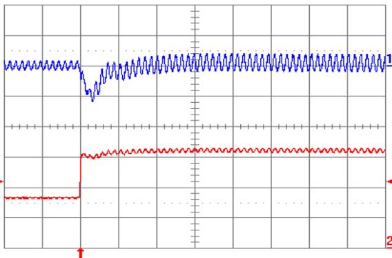
**Fig. 1.5V.7:** Output voltage response for  $V_{out} = 1.5\text{ V}$  to positive load current step change from  $2.5\text{ A}$  to  $5\text{ A}$  with slew rate of  $5\text{ A}/\mu\text{s}$  at  $V_{in} = 5\text{ V}$ . Top trace: output voltage ( $100\text{ mV/div.}$ ); Bottom trace: load current ( $2\text{ A/div.}$ ).  $C_o = 47\ \mu\text{F}$  ceramic +  $1\ \mu\text{F}$  ceramic. Time scale:  $20\ \mu\text{s/div.}$
