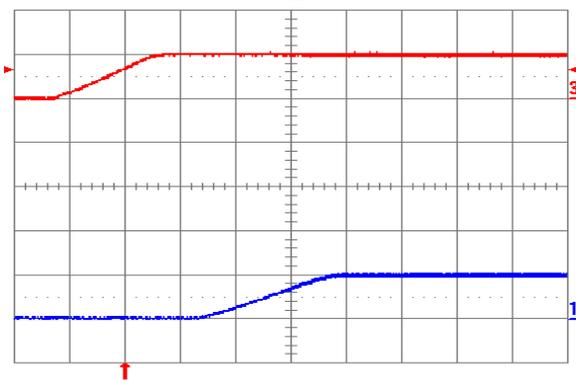
**Fig. 1.0V.5:** Turn-on transient for  $V_{out} = 1.0$  V with application of  $V_{in}$  at full rated load current (resistive) and  $47 \mu\text{F}$  external capacitance at  $V_{in} = 5$  V. Top trace:  $V_{in}$  (5 V/div.); Bottom trace: output voltage (1 V/div.); Time scale: 2 ms/div.
