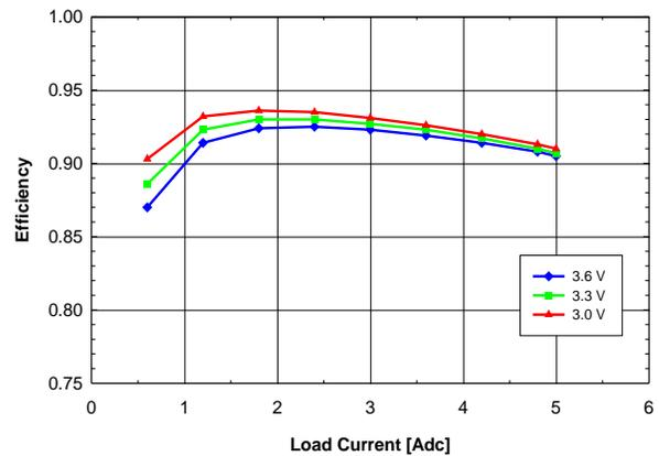
**Fig. 1.8V.4:** Efficiency vs. load current and input voltage for  $V_{out} = 1.8\text{ V}$  converter mounted horizontally with air flowing from pin 5 to pin 1 at a rate of 200 LFM (1 m/s) and  $T_a = 25\text{ }^{\circ}\text{C}$ .
