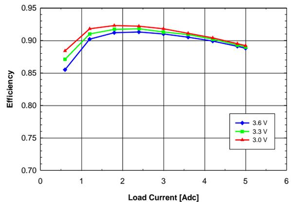
**Fig. 1.5V.4:** Efficiency vs. load current and input voltage for  $V_{out} = 1.5V$  converter mounted vertically with air flowing from pin 5 to pin 1 at a rate of 200 LFM (1 m/s) and  $T_a = 25^\circ C$ .
