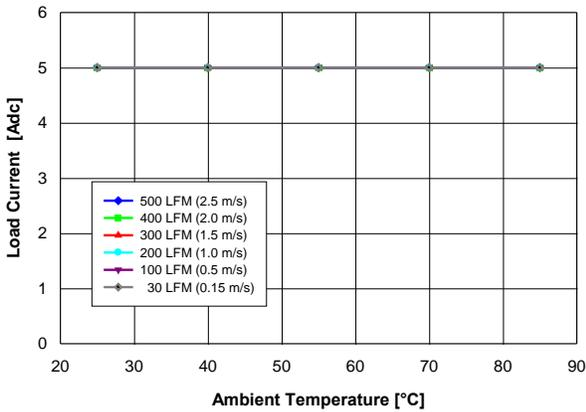
**Fig. 1.5V.1:** Available load current vs. ambient temperature and airflow rates for  $V_{out} = 1.5V$  converter mounted vertically with  $V_{in} = 5V$ , air flowing from pin 5 to pin 1 and maximum MOSFET temperature  $\leq 120^\circ C$ .
