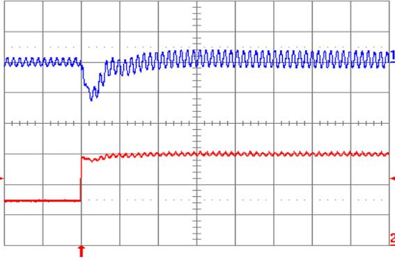
**Fig. 1.8V.7:** Output voltage response for  $V_{out} = 1.8V$  to positive load current step change from 2.5 A to 5 A with slew rate of  $5 A/\mu s$  at  $V_{in} = 5 V$ . Top trace: output voltage (100 mV/div.); Bottom trace: load current (2 A/div.).  $C_o = 47 \mu F$  ceramic +  $1 \mu F$  ceramic. Time scale:  $20 \mu s/div.$
