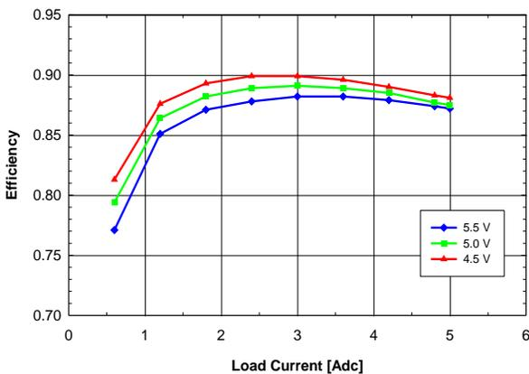
**Fig. 1.5V.3:** Efficiency vs. load current and input voltage for  $V_{out} = 1.5V$  converter mounted vertically with air flowing from pin 5 to pin 1 at a rate of 200 LFM (1 m/s) and  $T_a = 25^\circ C$ .
