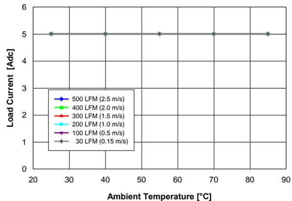
**Fig. 0.7525V.2:** Available load current vs. ambient temperature and airflow rates for  $V_{out} = 0.7525\text{ V}$  converter mounted horizontally with  $V_{in} = 5\text{ V}$ , air flowing from pin 5 to pin 1 and maximum MOSFET temperature  $\leq 120\text{ }^\circ\text{C}$ .
