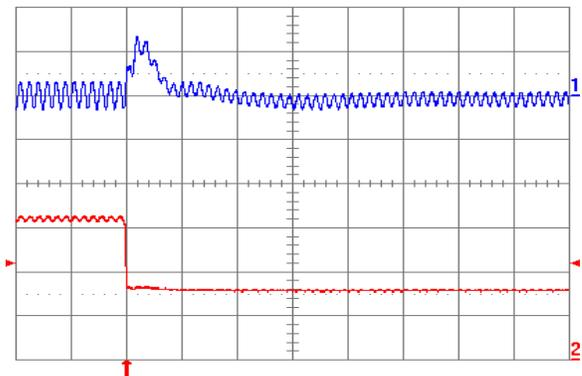
**Fig. 2.5V.8:** Output voltage response for  $V_{out} = 2.5\text{ V}$  to negative load current step change from  $5\text{ A}$  to  $2.5\text{ A}$  with slew rate of  $-5\text{ A}/\mu\text{s}$  at  $V_{in} = 5\text{ V}$ . Top trace: output voltage ( $100\text{ mV/div.}$ ); Bottom trace: load current ( $2\text{ A/div.}$ ).  $C_o = 47\ \mu\text{F}$  ceramic +  $1\ \mu\text{F}$  ceramic. Time scale:  $20\ \mu\text{s/div.}$
