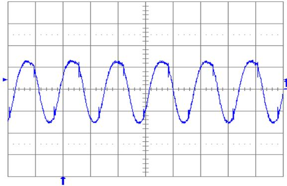
**Fig. 2.5V.5:** Output voltage ripple ( $20\text{ mV/div.}$ ) at full rated load current into a resistive load with external capacitance  $10\ \mu\text{F}$  ceramic +  $1\ \mu\text{F}$  ceramic and  $V_{in} = 5\text{ V}$  for  $V_{out} = 2.5\text{ V}$ . Time scale:  $2\ \mu\text{s/div.}$
