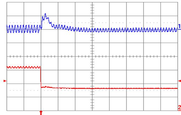
**Fig. 1.5V.8:** Output voltage response for  $V_{out} = 1.5\text{ V}$  to negative load current step change from  $5\text{ A}$  to  $2.5\text{ A}$  with slew rate of  $-5\text{ A}/\mu\text{s}$  at  $V_{in} = 5\text{ V}$ . Top trace: output voltage ( $100\text{ mV/div.}$ ); Bottom trace: load current ( $2\text{ A/div.}$ ).  $C_o = 47\ \mu\text{F}$  ceramic +  $1\ \mu\text{F}$  ceramic. Time scale:  $20\ \mu\text{s/div.}$
