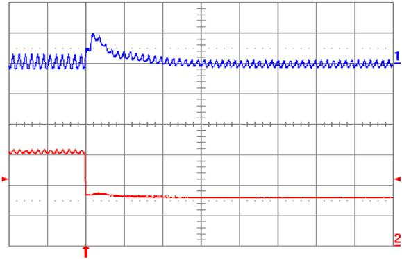
**Fig. 1.0V.8:** Output voltage response for  $V_{out} = 1.0\text{ V}$  to negative load current step change from 5 A to 2.5 A with slew rate of  $-5\text{ A}/\mu\text{s}$  at  $V_{in} = 5\text{ V}$ . Top trace: output voltage (100 mV/div.); Bottom trace: load current (2 A/div.).  $C_o = 47\text{ }\mu\text{F}$  ceramic +  $1\text{ }\mu\text{F}$  ceramic. Time scale:  $20\text{ }\mu\text{s}/\text{div}$ .
