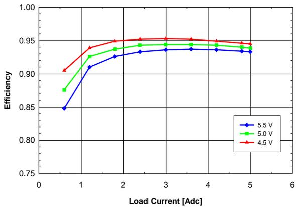
**Fig. 3.3V.3:** Efficiency vs. load current and input voltage for  $V_{out} = 3.3\text{ V}$  converter mounted vertically with air flowing from pin 5 to pin 1 at a rate of 200 LFM (1 m/s) and  $T_a = 25^\circ\text{C}$ .
