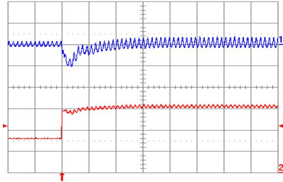
**Fig. 1.0V.7:** Output voltage response for  $V_{out} = 1.0\text{ V}$  to positive load current step change from 2.5 A to 5 A with slew rate of  $5\text{ A}/\mu\text{s}$  at  $V_{in} = 5\text{ V}$ . Top trace: output voltage (100 mV/div.); Bottom trace: load current (2 A/div.).  $C_o = 47\text{ }\mu\text{F}$  ceramic +  $1\text{ }\mu\text{F}$  ceramic. Time scale:  $20\text{ }\mu\text{s}/\text{div}$ .
