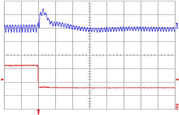
**Fig. 3.3V.8:** Output voltage response for  $V_{out} = 3.3\text{ V}$  to negative load current step change from 5 A to 2.5 A with slew rate of  $-5\text{ A}/\mu\text{s}$  at  $V_{in} = 5\text{ V}$ . Top trace: output voltage (100 mV/div.); Bottom trace: load current (2 A/div.).  $C_o = 47\text{ }\mu\text{F}$  ceramic +  $1\text{ }\mu\text{F}$  ceramic. Time scale:  $20\text{ }\mu\text{s}/\text{div}$ .
