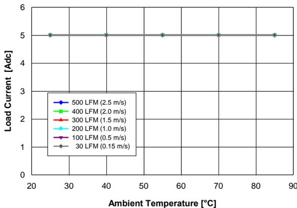
**Fig. 0.7525V.1:** Available load current vs. ambient temperature and airflow rates for  $V_{out} = 0.7525\text{ V}$  converter mounted vertically with  $V_{in} = 5\text{ V}$ , air flowing from pin 5 to pin 1 and maximum MOSFET temperature  $\leq 120\text{ }^\circ\text{C}$ .
