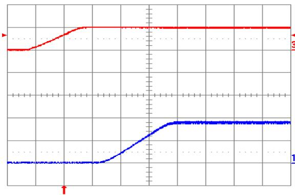
**Fig. 1.8V.5:** Turn-on transient for  $V_{out} = 1.8\text{ V}$  with application of  $V_{in}$  at full rated load current (resistive) and  $47\text{ }\mu\text{F}$  external capacitance at  $V_{in} = 5\text{ V}$ . Top trace:  $V_{in}$  (5 V/div.); Bottom trace: output voltage (1 V/div.); Time scale: 2 ms/div.
