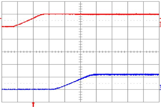
**Fig. 1.2V.5:** Turn-on transient for  $V_{out} = 1.2\text{ V}$  with application of  $V_{in}$  at full rated load current (resistive) and  $47\text{ }\mu\text{F}$  external capacitance at  $V_{in} = 5\text{ V}$ . Top trace:  $V_{in}$  (5 V/div.); Bottom trace: output voltage (1 V/div.); Time scale: 2 ms/div.
