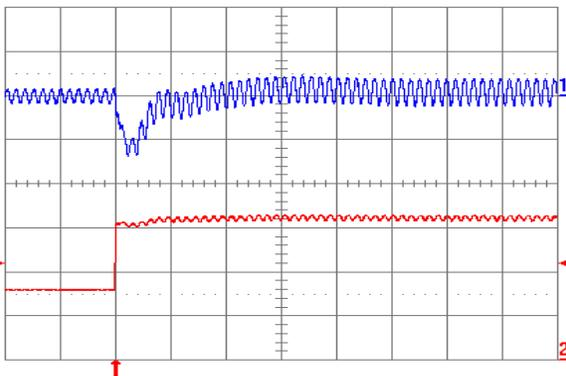
**Fig. 2.5V.7:** Output voltage response for  $V_{out} = 2.5\text{ V}$  to positive load current step change from  $2.5\text{ A}$  to  $5\text{ A}$  with slew rate of  $5\text{ A}/\mu\text{s}$  at  $V_{in} = 5\text{ V}$ . Top trace: output voltage ( $100\text{ mV/div.}$ ); Bottom trace: load current ( $2\text{ A/div.}$ ).  $C_o = 47\ \mu\text{F}$  ceramic +  $1\ \mu\text{F}$  ceramic. Time scale:  $20\ \mu\text{s/div.}$
