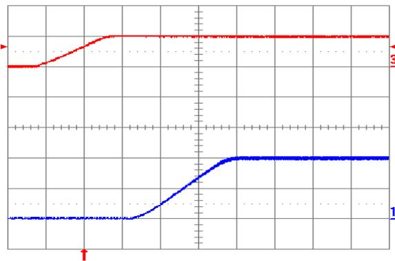
**Fig. 2.0V.5:** Turn-on transient for  $V_{out} = 2.0\text{ V}$  with application of  $V_{in}$  at full rated load current (resistive) and 47  $\mu\text{F}$  external capacitance at  $V_{in} = 5\text{ V}$ . Top trace:  $V_{in}$  (5 V/div.); Bottom trace: output voltage (1 V/div.); Time scale: 2 ms/div.
