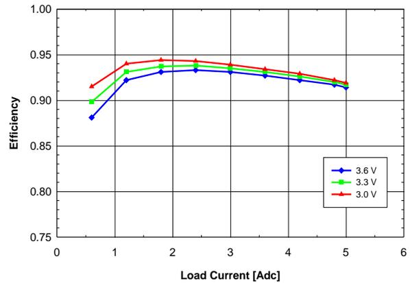
**Fig. 2.0V.4:** Efficiency vs. load current and input voltage for  $V_{out} = 2.0\text{ V}$  converter mounted vertically with air flowing from pin 5 to pin 1 at a rate of 200 LFM (1 m/s) and  $T_a = 25^\circ\text{C}$ .
