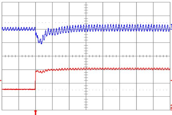
**Fig. 1.2V.7:** Output voltage response for  $V_{out} = 1.2\text{ V}$  to positive load current step change from 2.5 A to 5 A with slew rate of  $5\text{ A}/\mu\text{s}$  at  $V_{in} = 5\text{ V}$ . Top trace: output voltage (100 mV/div.); Bottom trace: load current (2 A/div.).  $C_o = 47\text{ }\mu\text{F}$  ceramic +  $1\text{ }\mu\text{F}$  ceramic. Time scale: 20  $\mu\text{s}$ /div.
