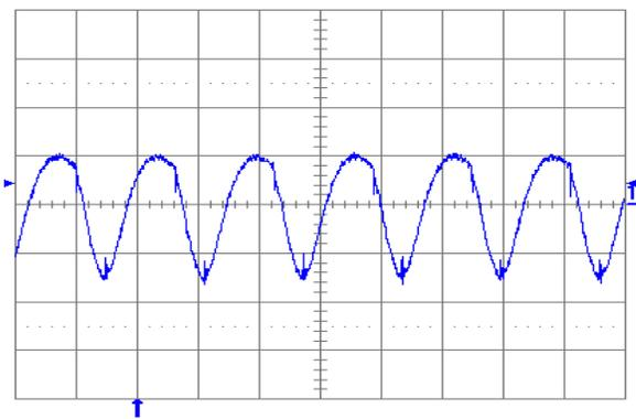
**Fig. 3.3V.6:** Output voltage ripple (20 mV/div.) at full rated load current into a resistive load with external capacitance  $10\ \mu\text{F}$  ceramic +  $1\ \mu\text{F}$  ceramic and  $V_{in} = 5\text{ V}$  for  $V_{out} = 3.3\text{ V}$ . Time scale: 2  $\mu\text{s}$ /div.
