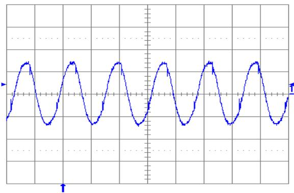
**Fig. 1.8V.6:** Output voltage ripple (20 mV/div.) at full rated load current into a resistive load with external capacitance  $10\text{ }\mu\text{F}$  ceramic +  $1\text{ }\mu\text{F}$  ceramic and  $V_{in} = 5\text{ V}$  for  $V_{out} = 1.8\text{ V}$ . Time scale: 2  $\mu\text{s}$ /div.
