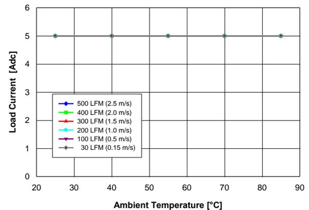
**Fig. 1.2V.2:** Available load current vs. ambient temperature and airflow rates for  $V_{out} = 1.2\text{ V}$  converter mounted horizontally with  $V_{in} = 5\text{ V}$ , air flowing from pin 5 to pin 1 and maximum MOSFET temperature  $\leq 120\text{ }^\circ\text{C}$ .
