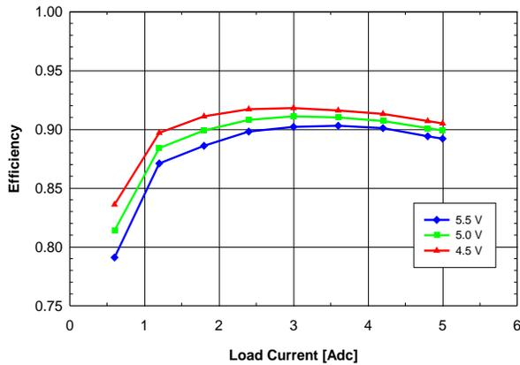
**Fig. 2.0V.3:** Efficiency vs. load current and input voltage for  $V_{out} = 2.0\text{ V}$  converter mounted vertically with air flowing from pin 5 to pin 1 at a rate of 200 LFM (1 m/s) and  $T_a = 25^\circ\text{C}$ .
