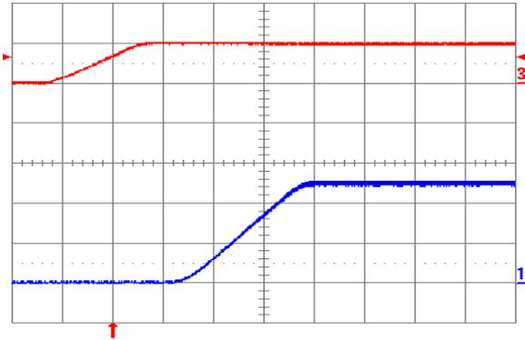
**Fig. 2.5V.4:** Turn-on transient for  $V_{out} = 2.5\text{ V}$  with application of  $V_{in}$  at full rated load current (resistive) and  $47\ \mu\text{F}$  external capacitance at  $V_{in} = 5\text{ V}$ . Top trace:  $V_{in}$  ( $5\text{ V/div.}$ ); Bottom trace: output voltage ( $1\text{ V/div.}$ ); Time scale:  $2\text{ ms/div.}$
