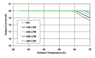
Figure 14. Derating Curves at Vo=1.2Vdc
