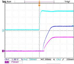
Figure 7. Typical Start-Up Using Remote On/Off (Vo = 3.3 Vdc, lo=20A). Ch1 – Vout, Ch2 – ON/OFF, Ch3 - lout
