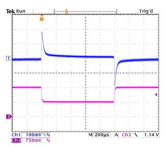
Figure 11.Transient Response to Dynamic Load Change from 50% to 100% of full load (Vin=12V, Vo=3.3Vdc). Ch3 – lout. Scale=10A/div
