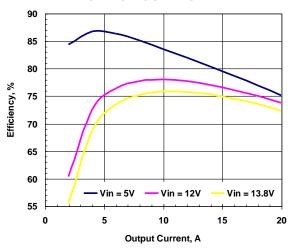
Figure 1. Efficiency vs. Load. Vout=0.6V
