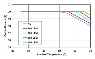
Figure 16. Derating Curves at Vo=2.5Vdc
