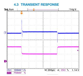
Figure 10.Transient Response to Dynamic Load Change from 50% to 100% of full load (Vin=12V, Vo=0.6Vdc). Ch3 – lout. Scale=10A/div
