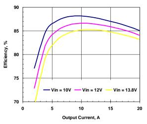
Figure 2. Efficiency vs. Load. Vout=1.2V
