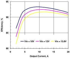
Figure 3. Efficiency vs. Load. Vout=2.5
