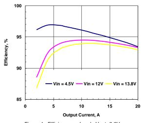
Figure 4. Efficiency vs. Load. Vout=3.3V
