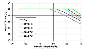
Figure 17. Derating Curves at Vo=3.3Vdc
