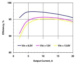
Figure 5. Efficiency vs. Load. Vout=5.0V
