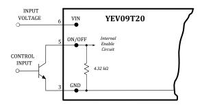
Figure 20. Circuit Configuration For ON/OFF Function
