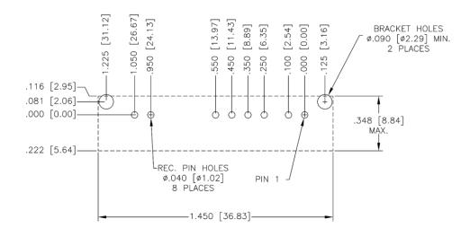
Figure 24. Recommended Footprint - Top View
