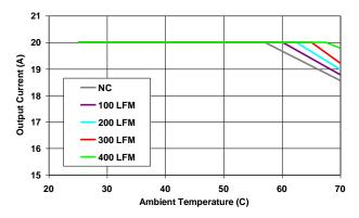
Figure 15. Derating Curves at Vo=1.8Vdc
