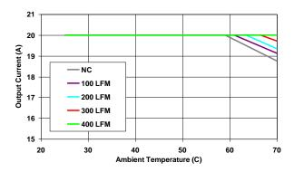
Figure 13. Derating Curves at Vo=0.9Vdc
