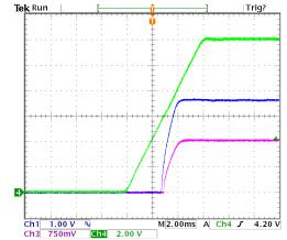
Figure 9. Typical Start-Up with application of Vin (Vo = 3.3Vdc, lo = 20A). Ch1 – Vout, Ch3 – lout, Ch4 – Vin,
