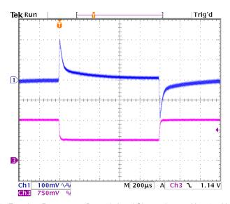
Figure 12. Transient Response to Dynamic Load Change from 50% to 100% of full load (Vin=12V, Vo=5.0Vdc). Ch3 – lout. Scale=10A/div
