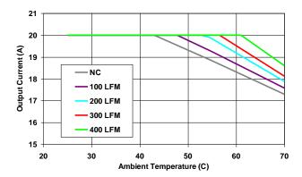
Figure 18. Derating Curves at Vo=5.0Vdc
