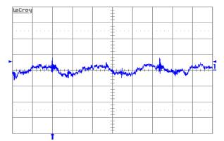
Figure 12. Input reflected-ripple current, is (10 mA/div.), measured through 10μH at the source at full rated load current and Vin = 48V. Refer to Figure 11 for test setup. Time scale: 1μs/div.
