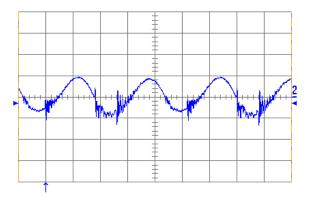
Figure 10. Output voltage ripple (20mV/div.) at full rated load current into a resistive load with Co = 10μF tantalum + 1μF ceramic and Vin = 48V. Time scale: 1μs/div.
