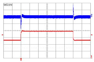
Figure 9. Output voltage response to load current step-change (12.5A–18.75A–12.5A) at Vin=48V. Top trace: output voltage (100 mV/div.). Bottom trace: load current (5A/div.). Current slew rate: 5A/µs. Co=470µF POS+1µF cer. Time scale: 0.2ms/div.
