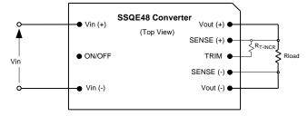
Figure C. Configuration for increasing output voltage.
