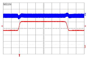
Figure 8. Output voltage response to load current step-change (12.5A–18.75A–12.5A) at Vin = 48V. Top trace: output voltage (100mV/div.). Bottom trace: load current (5A/div.). Current slew rate: 0.1A/µs. Co=1µF cer+10µF tant. Time scale: 0.2ms/div.
