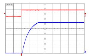
Figure 7. Turn-on transient at full rated load current (resistive) plus 10,000 µF at Vin = 48 V, triggered via ON/OFF pin. Top trace: ON/OFF signal (5 V/div.). Bottom trace: Output voltage (1 V/div.). Time scale: 5 ms/div.
