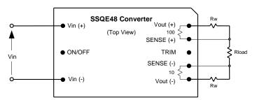
Figure B. Remote sense circuit configuration.
