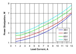
Figure 4. Power dissipation vs. load current and input voltage for SSQE48T13050 converter mounted vertically with air flowing from pin 1 to pin 3 at a rate of 300 LFM (1.5 m/s) and Ta = 25°C
