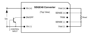
Figure A. Circuit configuration for ON/OFF function.
