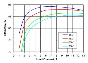
Figure 2. Efficiency vs. load current and input voltage for SSQE48T13050 converter mounted vertically with air flowing from pin 1 to pin 3 at a rate of 300 LFM (1.5 m/s) and Ta = 25°C.
