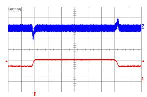
Figure 8. Output voltage response to load current step-change (6.5 A–9.75 A–6.5 A) at Vin = 48 V. Top trace: output voltage (100 mV/div.). Bottom trace: load current (5 A/div.).
