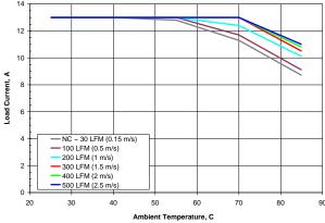
Figure 1. Available load current vs. ambient air temperature and airflow rates for SSQE48T13050 converter mounted vertically with air flowing from pin 1 to pin 3, Vin = 48 V.
