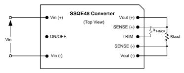
Figure C. Configuration for increasing output voltage.
