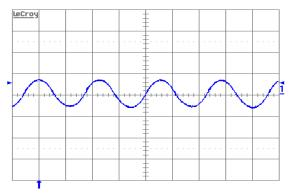
Figure 13. Input reflected ripple-current, i<sub>c</sub> (200 mA/div.), measured at input terminals at full rated load current and Vin = 48 V. Refer to Figure 11 for test setup. Time scale: 1 μs/div.
