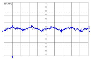
Figure 12. Input reflected-ripple current, i<sub>s</sub> (10 mA/div.), measured through 10 μH at the source at full rated load current and Vin = 48V. Refer to Figure 11 for test setup. Time scale: 1 μs/div.
