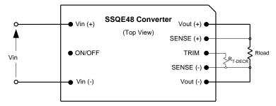
Figure D. Configuration for decreasing output voltage.
