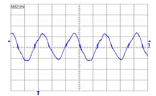
Figure 10. Output voltage ripple (20 mV/div.) at full rated load current into a resistive load with Co = 10 μF tantalum + 1 μF ceramic and Vin = 48 V. Time scale: 1 μs/div.
