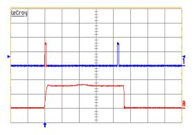
Figure 15. Load current (top trace, 10 A/div., 50 ms/div.) into a 10mΩ short circuit during restart, at Vin = 48 V. Bottom trace (10A/div., 1.0ms/div.) is an expansion of the on-time portion of the top trace.
