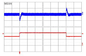
Figure 9. Output voltage response to load current step-change (6.5 A-9.75 A-6.5 A) at Vin = 48 V. Top trace: output voltage (100 mV/div.). Bottom trace: load current (5A/div.). Current slew rate: 5 A/µs. Co= 470 µF POS + 1µF ceramic.
