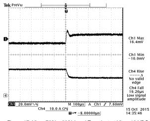
Figure 17. Vin = 75% - 50% Load Transient at Vin = 12 VDC Vout = 0.9 VDC @ Ta = 25℃
