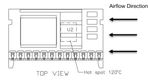
Figure 7. Airflow direction, Hot spot location and allowed maximum temperature
