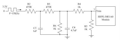
Figure 29. Trim up circuit (using external PWM signal)
