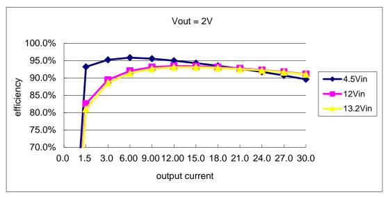
Figure 3. Efficiency @ Vo = 2.0 V
