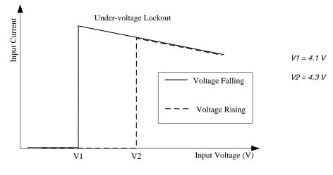
Figure 20. Input under-voltage lockout
