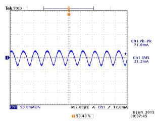
Figure 5. is (input terminal ripple current), AC component
