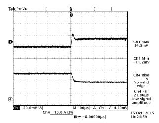
Figure 15. Vin = 75% - 50% Load Transient at Vin = 12 VDC Vout = 0.6 VDC @ Ta = 25°C
