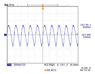
Figure 6. ic (input terminal ripple current), AC component
