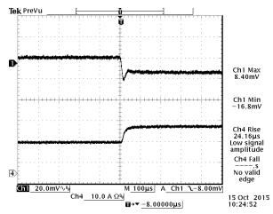
Figure 14. Vin = 50%-75% Load Transient at Vin = 12 VDC Vout = 0.6 VDC @ Ta = 25℃
