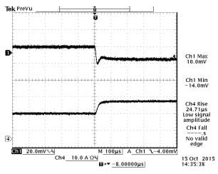
Figure 16. Vin = 50%-75% Load Transient at Vin = 12 VDC Vout = 0.9 VDC @ Ta = 25℃
