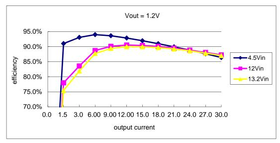
Figure 2. Efficiency @ Vo = 1.2 V
