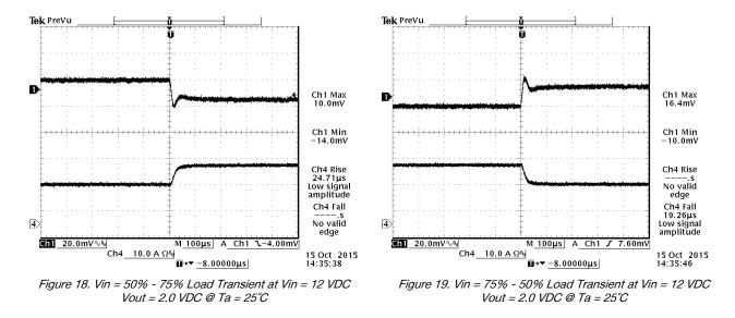
**NOTE**: Test condition of the Transient response:  $di/dt = 2.5 \text{ A/}\mu\text{s}$ , with a 10  $\mu\text{F}$ +7\*100  $\mu\text{F}$  ceramic cap and 3\*470  $\mu\text{F}$  POSCAP ESR  $\leq$  12 m ohm at output.
