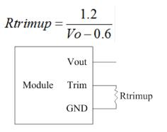
Figure 27. Trim up circuit (using an external resistor)
