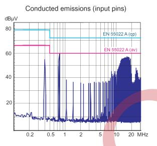
To meet level B, it is necessary to fit a 5 µF ceramic capacitor across the input terminals.
