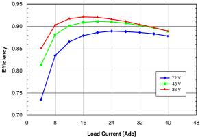
Figure 2.5V.11. Efficiency vs. load current and input voltage for QME48T40025 converter mounted horizontally with air flowing from pin 1 to pin 3 at a rate of 300 LFM (1.5 m/s) and Ta = 25 °C.
