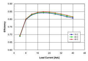
Figure 1.2V.12. Efficiency vs. load current and ambient temperature for QME48T40012 converter mounted horizontally with Vin = 48 V and air flowing from pin 1 to pin 3 at a rate of 200 LFM (1.0 m/s).
