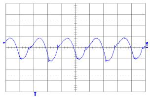
Figure 1.5V.19. Output voltage ripple (20 mV/div.) at full rated load current into a resistive load with Co = 10 μF tantalum + 1 μF ceramic and Vin = 48 V. Time scale: 1 μs/div.
