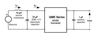
Figure 1.8V.20. Test setup for measuring input reflected ripple currents, ic and is.
