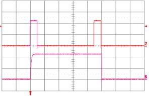
Figure 1.0V.24. Load current (top trace, 20 A/div., 50 ms/div.) into a 10 mΩ short circuit during restart, at Vin = 48 V. Bottom trace (20 A/div., 5 ms/div.) is an expansion of the on-time portion of the top trace.
