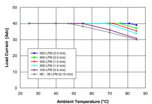
Figure 1.0V.9. Available load current vs. ambient air temperature and airflow rates for QME48T40010 converter with G height pins mounted vertically with air flowing from pin 1 to pin 3, MOSFET temperature ≤ 120 °C, Vin = 48 V.
