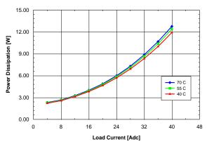
Figure 1.8V.14. Power dissipation vs. load current and ambient temperature for QME48T40018 converter mounted horizontally with Vin = 48 V and air flowing from pin 1 to pin 3 at a rate of 200 LFM (1.0 m/s).
