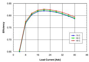
Figure 1.0V.12. Efficiency vs. load current and ambient temperature for QME48T40010 converter mounted horizontally with Vin = 48 V and air flowing from pin 1 to pin 3 at a rate of 200 LFM (1.0 m/s).
