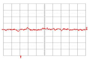
Figure 1.0V.22. Input reflected ripple current, is (10 mA/div.), measured through 10 µH at the source at full rated load current and Vin = 48 V. Refer to Fig. 1.0V.20 for test setup. Time scale: 1 µs/div.
