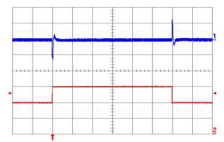
Figure 1.8V.18. Output voltage response to load current stepchange (20 A – 30 A – 20 A) at Vin = 48 V. Top trace: output voltage (100 mV/div.). Bottom trace: load current (10 A/div.). Current slew rate: 5 A/μs. Co = 470 μF POS + 1 μF ceramic. Time scale: 0.2 ms/div.
