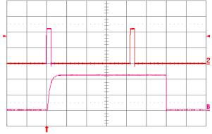
Figure 1.8V.24. Load current (top trace, 20 A/div., 50 ms/div.) into a 10 mΩ short circuit during restart, at Vin = 48 V. Bottom trace (20 A/div., 2 ms/div.) is an expansion of the on-time portion of the top trace.
