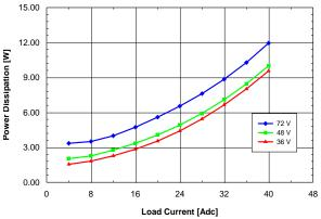
Figure 1.0V.13. Power dissipation vs. load current and input voltage for QME48T40010 converter mounted horizontally with air flowing from pin 1 to pin 3 at a rate of 300 LFM (1.5 m/s) and Ta = 25 °C.
