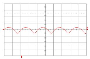
Figure 1.0V.21. Input reflected ripple current, ic (100 mA/div.), measured at input terminals at full rated load current and Vin = 48 V. Refer to Fig. 1.0V.20 for test setup.
