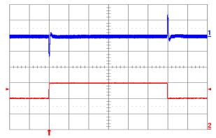
Figure 2.5V.18. Output voltage response to load current stepchange (20 A – 30 A – 20 A) at Vin = 48 V. Top trace: output voltage (100 mV/div.). Bottom trace: load current (10 A/div.). Current slew rate: 5A/μs. Co = 470 μF POS + 1 μF ceramic. Time scale: 0.2 ms/div.
