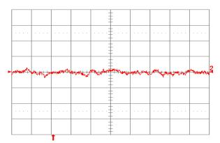
Figure 1.2V.22. Input reflected ripple current, is (10 mA/div.), measured through 10 µH at the source at full rated load current and Vin = 48 V. Refer to Fig. 1.2V.20 for test setup. Time scale: 1 µs/div.
