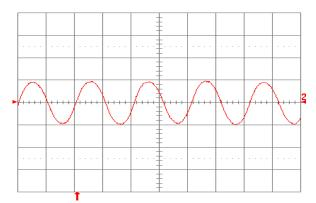
Figure 2.5V.21. Input reflected ripple current, ic (100 mA/div.), measured at input terminals at full rated load current and Vin = 48 V. Refer to Fig. 2.5V.20 for test setup.
