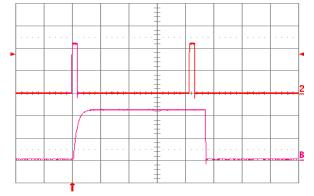
Figure 2.5V.24. Load current (top trace, 20 A/div., 50 ms/div.) into a 10 mΩ short circuit during restart, at Vin = 48 V. Bottom trace (20 A/div., 2 ms/div.) is an expansion of the on-time portion of the top trace.
