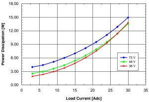
Figure 3.3V.13. Power dissipation vs. load current and input voltage for QME48T40033 converter mounted horizontally with air flowing from pin 1 to pin 3 at a rate of 300 LFM (1.5 m/s) and Ta = 25 °C.
