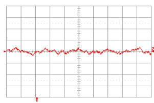
Figure 2.5V.22. Input reflected ripple current, is (10 mA/div.), measured through 10 µH at the source at full rated load current and Vin = 48 V. Refer to Fig. 2.5V.20 for test setup. Time scale: 1 µs/div.
