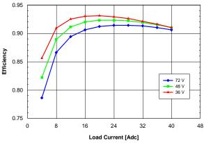
Figure 3.3V.11. Efficiency vs. load current and input voltage for QME48T40033 converter mounted horizontally with air flowing from pin 1 to pin 3 at a rate of 300 LFM (1.5 m/s) and Ta = 25 °C.
