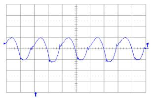
Figure 1.8V.19. Output voltage ripple (20mV/div.) at full rated load current into a resistive load with Co = 10 μF tantalum + 1 μF ceramic and Vin = 48 V. Time scale: 1 μs/div.
