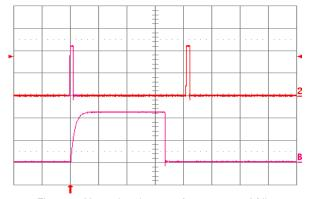
Figure 3.3V.24. Load current (top trace, 20 A/div., 50 ms/div.) into a 10 mΩ short circuit during restart, at Vin = 48 V. Bottom trace (20 A/div., 2 ms/div.) is an expansion of the on-time portion of the top trace.
