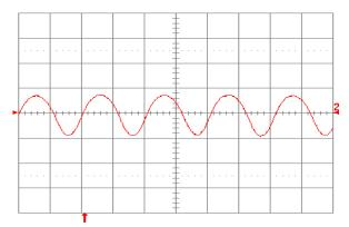
Figure 1.8V.21. Input reflected ripple current, ic (100 mA/div.), measured at input terminals at full rated load current and Vin = 48 V. Refer to Fig. 1.8V.20 for test setup.
