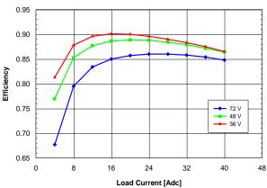
Figure 1.8V.11. Efficiency vs. load current and input voltage for QME48T40018 converter mounted horizontally with air flowing from pin 1 to pin 3 at a rate of 300 LFM (1.5 m/s) and Ta = 25 °C.
