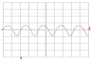
Figure 1.5V.21. Input reflected ripple current, ic (100 mA/div.), measured at input terminals at full rated load current and Vin = 48 V. Refer to Fig. 1.5V.20 for test setup.
