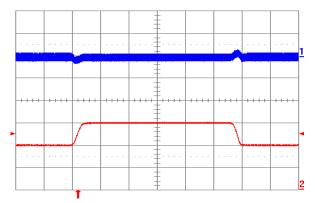
Figure 1.5V.17. Output voltage response to load current stepchange (20 A – 30 A – 20 A) at Vin = 48 V. Top trace: output voltage (100 mV/div.). Bottom trace: load current (10 A/div.). Current slew rate: 0.1 A/μs. Co = 1 μF ceramic. Time scale: 0.2 ms/div.
