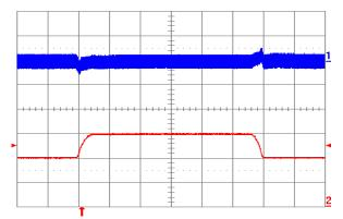
Figure 3.3V.17. Output voltage response to load current stepchange (20 A – 30 A – 20 A) at Vin = 48 V. Top trace: output voltage (100 mV/div.). Bottom trace: load current (10 A/div.). Current slew rate: 0.1 A/μs. Co = 1 μF ceramic. Time scale: 0.2 ms/div.
