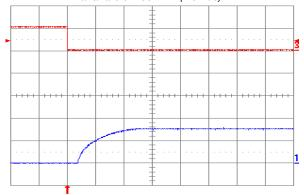
Figure 1.5V.16. Turn-on transient at full rated load current (resistive) plus 10,000 µF at Vin = 48 V, triggered via ON/OFF pin. Top trace: ON/OFF signal (5 V/div.). Bottom trace: output voltage (1 V/div.). Time scale: 2 ms/div.
