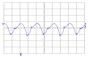
Figure 1.2V.19. Output voltage ripple (20 mV/div.) at full rated load current into a resistive load with Co = 10 μF tantalum + 1 μF ceramic and Vin = 48 V. Time scale: 1 μs/div.
