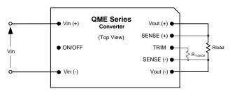
Figure 4. Configuration for decreasing output voltage.
