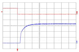
Figure 3.3V.15. Turn-on transient at full rated load current (resistive) with no output capacitor at Vin = 48 V, triggered via ON/OFF pin. Top trace: ON/OFF signal (5 V/div.). Bottom trace: output voltage (1 V/div.). Time scale: 2 ms/div.
