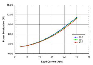
Figure 1.2V.14. Power dissipation vs. load current and ambient temperature for QME48T40012 converter mounted horizontally with Vin = 48 V and air flowing from pin 1 to pin 3 at a rate of 200 LFM (1.0 m/s).
