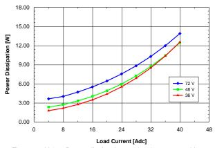
Figure 2.5V.13. Power dissipation vs. load current and input voltage for QME48T40025 converter mounted horizontally with air flowing from pin 1 to pin 3 at a rate of 300 LFM (1.5 m/s) and Ta = 25 °C.
