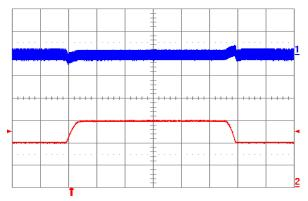
Figure 2.5V.17. Output voltage response to load current stepchange (20 A – 30 A – 20 A) at Vin = 48 V. Top trace: output voltage (100 mV/div.). Bottom trace: load current (10 A/div.). Current slew rate: 0.1 A/μs. Co = 1 μF ceramic. Time scale: 0.2 ms/div.
