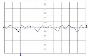
Figure 1.0V.18. Output voltage response to load current stepchange (20 A – 30 A – 20 A) at Vin = 48 V. Top trace: output voltage (100 mV/div.). Bottom trace: load current (10 A/div.). Current slew rate: 5 A/μs. Co = 470 μF POS + 1 μF ceramic. Time scale: 0.2 ms/div.
