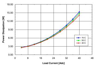
Figure 3.3V.14. Power dissipation vs. load current and ambient temperature for QME48T40033 converter mounted horizontally with Vin = 48 V and air flowing from pin 1 to pin 3 at a rate of 200 LFM (1.0 m/s).
