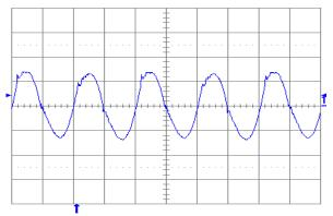
Figure 3.3V.19. Output voltage ripple (20 mV/div.) at full rated load current into a resistive load with Co = 10 μF tantalum + 1 μF ceramic and Vin = 48 V. Time scale: 1 μs/div.
