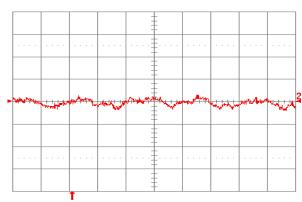
Figure 3.3V.22. Input reflected ripple current, is (10 mA/div.), measured through 10 µH at the source at full rated load current and Vin = 48 V. Refer to Fig. 3.3V.20 for test setup. Time scale: 1 µs/div.
