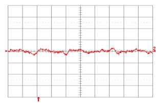
Figure 1.8V.22. Input reflected ripple current, is (10 mA/div.), measured through 10 µH at the source at full rated load current and Vin = 48 V. Refer to Fig. 1.8V.20 for test setup. Time scale: 1 µs/div.
