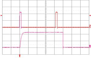
Figure 1.5V.24. Load current (top trace, 20 A/div., 50 ms/div.) into a 10 mΩ short circuit during restart, at Vin = 48 V. Bottom trace (20 A/div., 2 ms/div.) is an expansion of the on-time portion of the top trace.
