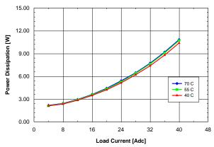
Figure 1.0V.14. Power dissipation vs. load current and ambient temperature for QME48T40010 converter mounted horizontally with Vin = 48 V and air flowing from pin 1 to pin 3 at a rate of 200 LFM (1.0 m/s).
