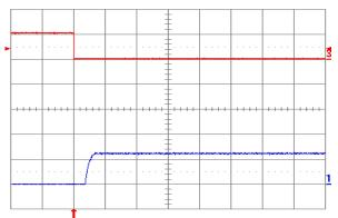
Figure 1.2V.15. Turn-on transient at full rated load current (resistive) with no output capacitor at Vin = 48 V, triggered via ON/OFF pin. Top trace: ON/OFF signal (5 V/div.). Bottom trace: output voltage (1 V/div.). Time scale: 2 ms/div.
