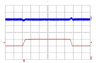
Figure 1.0V.17. Output voltage response to load current stepchange (20 A – 30 A – 20 A) at Vin = 48 V. Top trace: output voltage (100 mV/div.). Bottom trace: load current (10 A/div.). Current slew rate: 0.1 A/µs. Co = 1 µF ceramic. Time scale: 0.2 ms/div.
