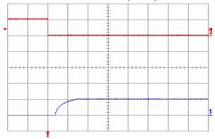
Figure 1.0V.16. Turn-on transient at full rated load current (resistive) plus 10,000 µF at Vin = 48 V, triggered via ON/OFF pin. Top trace: ON/OFF signal (5 V/div.). Bottom trace: output voltage (1 V/div.). Time scale: 2 ms/div.
