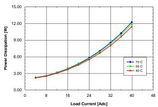
Figure 1.5V.14. Power dissipation vs. load current and ambient temperature for QME48T40015 converter mounted horizontally with Vin = 48 V and air flowing from pin 1 to pin 3 at a rate of 200 LFM (1.0 m/s).
