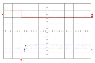
Figure 1.0V.15. Turn-on transient at full rated load current (resistive) with no output capacitor at Vin = 48 V, triggered via ON/OFF pin. Top trace: ON/OFF signal (5 V/div.). Bottom trace: output voltage (1 V/div.). Time scale: 2 ms/div
