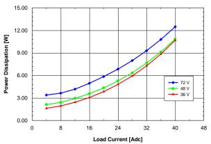
Figure 1.5V.13. Power dissipation vs. load current and input voltage for QME48T40015 converter mounted horizontally with air flowing from pin 1 to pin 3 at a rate of 300 LFM (1.5 m/s) and Ta = 25 °C.
