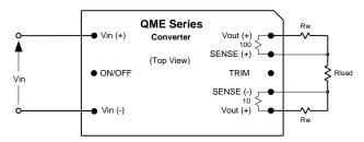
Figure 2. Remote sense circuit configuration
