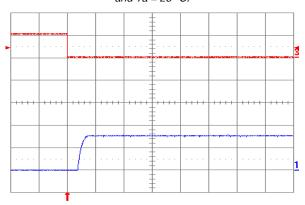
Figure 1.5V.15. Turn-on transient at full rated load current (resistive) with no output capacitor at Vin = 48 V, triggered via ON/OFF pin. Top trace: ON/OFF signal (5 V/div.). Bottom trace: output voltage (1 V/div.). Time scale: 2 ms/div.
