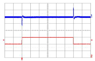
Figure 3.3V.18. Output voltage response to load current stepchange (20 A – 30 A – 20 A) at Vin = 48 V. Top trace: output voltage (100 mV/div.). Bottom trace: load current (10 A/div.). Current slew rate: 5 A/μs. Co = 470 μF POS + 1 μF ceramic. Time scale: 0.2 ms/div.
