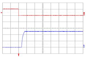
Figure 2.5V.15. Turn-on transient at full rated load current (resistive) with no output capacitor at Vin = 48 V, triggered via ON/OFF pin. Top trace: ON/OFF signal (5 V/div.). Bottom trace: output voltage (1 V/div.). Time scale: 2 ms/div.
