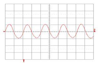
Figure 3.3V.21. Input reflected ripple current, ic (100 mA/div.), measured at input terminals at full rated load current and Vin = 48 V. Refer to Fig. 3.3V.20 for test setup.
