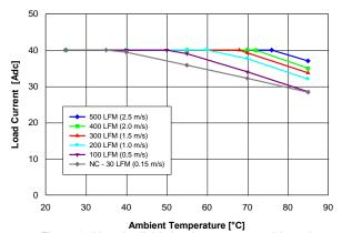
Figure 1.8V.9. Available load current vs. ambient air temperature and airflow rates for QME48T40018 converter with G height pins mounted vertically with air flowing from pin 1 to pin 3, MOSFET temperature ≤ 120 °C, Vin = 48 V.
