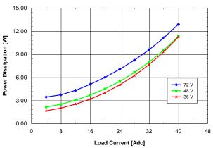
Figure 1.8V.13. Power dissipation vs. load current and input voltage for QME48T40018 converter mounted horizontally with air flowing from pin 1 to pin 3 at a rate of 300 LFM (1.5 m/s) and Ta = 25 °C.
