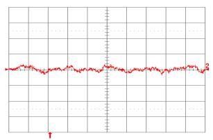
Figure 1.5V.22. Input reflected ripple current, is (10 mA/div.), measured through 10 µH at the source at full rated load current and Vin = 48 V. Refer to Fig. 1.5V.20 for test setup. Time scale: 1 µs/div..
