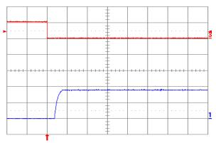
Figure 1.8V.15. Turn-on transient at full rated load current (resistive) with no output capacitor at Vin = 48 V, triggered via ON/OFF pin. Top trace: ON/OFF signal (5 V/div.). Bottom trace: output voltage (1 V/div.). Time scale: 2 ms/div.
