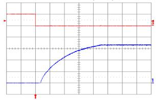
Figure 3.3V.16. Turn-on transient at full rated load current (resistive) plus 10,000 μF at Vin = 48 V, triggered via ON/OFF pin. Top trace: ON/OFF signal (5 V/div.). Bottom trace: output voltage (1 V/div.). Time scale: 2 ms/div.
