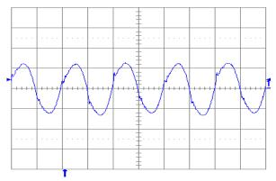
Figure 2.5V.19. Output voltage ripple (20 mV/div.) at full rated load current into a resistive load with Co = 10 μF tantalum + 1 μF ceramic and Vin = 48 V. Time scale: 1 μs/div.
