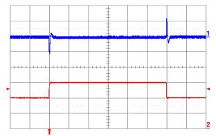
Figure 1.5V.18. Output voltage response to load current stepchange (20 A – 30 A – 20 A) at Vin = 48 V. Top trace: output voltage (100 mV/div.). Bottom trace: load current (10 A/div.). Current slew rate: 5A/μs. Co = 470 μF POS + 1 μF ceramic. Time scale: 0.2 ms/div.
