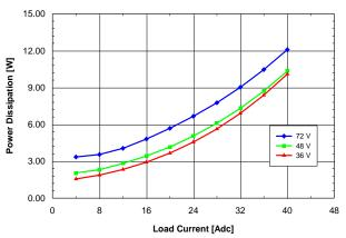
Figure 1.2V.13. Power dissipation vs. load current and input voltage for QME48T40012 converter mounted horizontally with air flowing from pin 1 to pin 3 at a rate of 300 LFM (1.5 m/s) and Ta = 25 °C.
