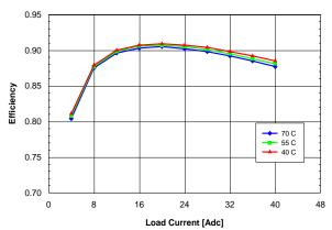
Figure 2.5V.12. Efficiency vs. load current and ambient temperature for QME48T40025 converter mounted horizontally with Vin = 48 V and air flowing from pin 1 to pin 3 at a rate of 200 LFM (1.0 m/s).
