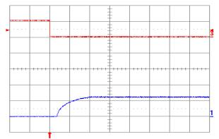
Figure 1.2V.16. Turn-on transient at full rated load current (resistive) plus 10,000 µF at Vin = 48 V, triggered via ON/OFF pin. Top trace: ON/OFF signal (5 V/div.). Bottom trace: output voltage (1 V/div.). Time scale: 2 ms/div.
