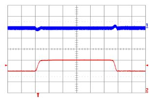
Figure 1.2V.17. Output voltage response to load current stepchange (20 A – 30 A – 20 A) at Vin = 48 V. Top trace: output voltage (100 mV/div.). Bottom trace: load current (10 A/div.). Current slew rate: 0.1 A/μs. Co = 1 μF ceramic. Time scale: 0.2 ms/div.
