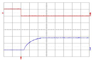
Figure 1.8V.16. Turn-on transient at full rated load current (resistive) plus 10,000 µF at Vin = 48 V, triggered via ON/OFF pin. Top trace: ON/OFF signal (5 V/div.). Bottom trace: output voltage (1 V/div.). Time scale: 2 ms/div.
