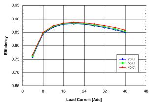
Figure 1.8V.12. Efficiency vs. load current and ambient temperature for QME48T40018 converter mounted horizontally with Vin = 48 V and air flowing from pin 1 to pin 3 at a rate of 200 LFM (1.0 m/s).
