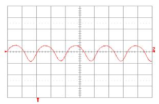
Figure 1.2V.21. Input reflected ripple current, ic (100 mA/div.), measured at input terminals at full rated load current and Vin = 48 V. Refer to Fig. 1.2V.20 for test setup. Time scale: 1 µs/div.
