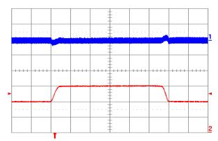
Figure 1.8V.17. Output voltage response to load current stepchange (20 A – 30 A – 20 A) at Vin = 48 V. Top trace: output voltage (100 mV/div.). Bottom trace: load current (10 A/div.). Current slew rate: 0.1 A/μs. Co = 1 μF ceramic. Time scale: 0.2 ms/div.
