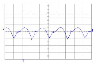
Figure 1.0V.19. Output voltage ripple (20 mV/div.) at full rated load current into a resistive load with  $Co = 10 \mu F$  tantalum + 1  $\mu F$  ceramic and Vin = 48 V. Time scale: 1  $\mu S/div$ .
