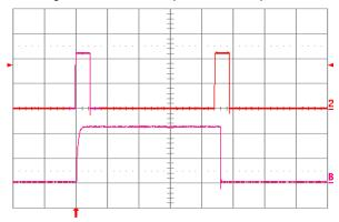
Figure 1.2V.24. Load current (top trace, 20 A/div., 50 ms/div.) into a 10 mΩ short circuit during restart, at Vin = 48 V. Bottom trace (20 A/div., 5 ms/div.) is an expansion of the on-time portion of the top trace.
