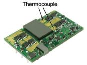
Figure 8. Location of the thermocouple for thermal testing.
