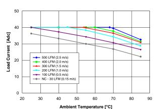
Figure 3.3V.10. Available load current vs. ambient air temperature and airflow rates for QME48T40033 converter with G height pins mounted horizontally with air flowing from pin 1 to pin 3, MOSFET temperature  $\leq$  120 °C, Vin = 48 V.
