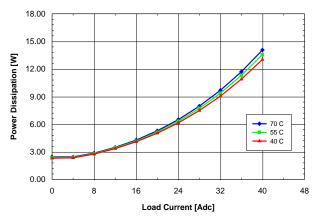
Figure 2.5V.14. Power dissipation vs. load current and ambient temperature for QME48T40025 converter mounted horizontally with Vin = 48 V and air flowing from pin 1 to pin 3 at a rate of 200 LFM (1.0 m/s).
