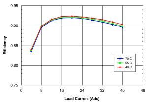
Figure 3.3V.12. Efficiency vs. load current and ambient temperature for QME48T40033 converter mounted horizontally with Vin = 48 V and air flowing from pin 1 to pin 3 at a rate of 200 LFM (1.0 m/s).
