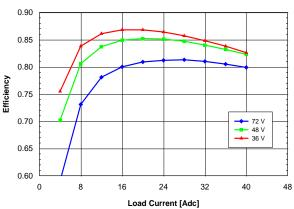
Figure 1.2V.11. Efficiency vs. load current and input voltage for QME48T40012 converter mounted horizontally with air flowing from pin 1 to pin 3 at a rate of 300 LFM (1.5 m/s) and Ta = 25 °C.
