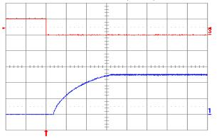
Figure 2.5V.16. Turn-on transient at full rated load current (resistive) plus 10,000 μF at Vin = 48 V, triggered via ON/OFF pin. Top trace: ON/OFF signal (5 V/div.). Bottom trace: output voltage (1 V/div.). Time scale: 2 ms/div.
