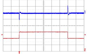
Figure 1.2V.18. Output voltage response to load current stepchange (20 A – 30 A – 20 A) at Vin = 48 V. Top trace: output voltage (100 mV/div.). Bottom trace: load current (10 A/div.). Current slew rate: 5 A/μs. Co = 470 μF POS + 1 μF ceramic. Time scale: 0.2 ms/div.
