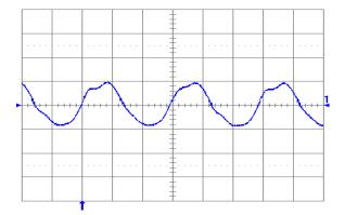
Figure 20. Output voltage ripple (20 mV/div.) at full rated load current into a resistive load with Co = 10 μF tantalum + 1uF ceramic and Vin = 48 V. Time scale: 1 μs/div.
