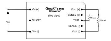
Figure 3. Configuration for increasing output voltage.
