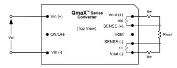
Figure 2. Remote sense circuit configuration
