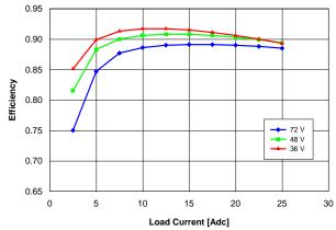
Figure 13. Efficiency vs. load current and input voltage for converter mounted vertically with air flowing from pin 3 to pin 1 at a rate of 300 LFM (1.5 m/s) and Ta = 25°C.
