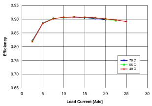
Figure 14. Efficiency vs. load current and ambient temperature for converter mounted vertically with Vin = 48 V and air flowing from pin 3 to pin 1 at a rate of 200 LFM (1.0 m/s).
