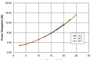
Load Current [Adc] Figure 16. Power dissipation vs. load current and ambient
