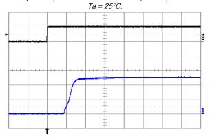
Figure 17. Turn-on transient at full rated load current (resistive) with no output capacitor at Vin = 48 V, triggered via ON/OFF pin. Top trace: ON/OFF signal (5 V/div.). Bottom trace: output voltage (2 V/div.) Time scale: 2 ms/div.
