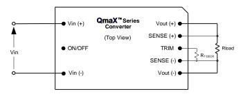
Figure 4. Configuration for decreasing output voltage.
