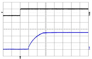
Figure 18. Turn-on transient at full rated load current (resistive) plus 10,000 μF at Vin = 48 V, triggered via ON/OFF pin. Top trace: ON/OFF signal (5 V/div.). Bottom trace: output voltage (2 V/div.). Time scale: 2 ms/div.
