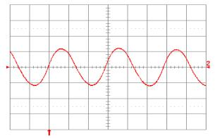
Figure 23. Input reflected ripple current, i<sub>c</sub> (200 mA/div), measured at input terminals at full rated load current and Vin = 48 V. Refer to Fig. 21 for test setup. Time scale: 1  $\mu$ s/div.
