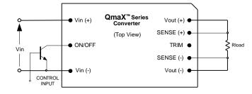
Figure 1. Circuit configuration for ON/OFF function.
