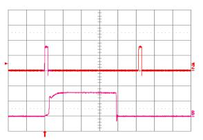
Figure 25. Load current (top trace, 20 A/div, 20 ms/div) into a 10 m $\Omega$  short circuit during restart, at Vin = 48 V. Bottom trace (20 A/div, 1 ms/div) is an expansion of the on-time portion of the top trace.
