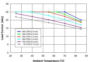
Figure 10. Available load current vs. ambient air temperature and airflow rates for QM48T25050 converter with B height pins mounted horizontally with air flowing from pin 3 to pin 1, MOSFET temperature ≤ 120°C, Vin = 48 V.
