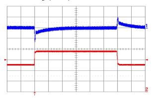
Figure 19. Output voltage response to load current stepchange (12.5 A – 18.75 A – 12.5 A) at Vin = 48 V. Top trace: output voltage (100 mV/div.). Bottom trace: load current (5 A/div). Current slew rate: 1 A/μs. Co = 470 μF tantalum + 1 μF ceramic. Time scale: 0.2 ms/div.
