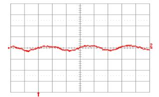
Figure 22. Input reflected ripple current, i<sub>s</sub> (10 mA/div), measured through 10 μH at the source at full rated load current and Vin = 48 V. Refer to Fig. 21 for test setup. Time scale: 1μs/div.
