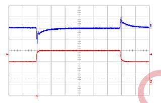
Fig. 9: Output voltage response to load current stepchange (20 A – 30 A – 20 A) at Vin = 48 V. Top trace: output voltage (100 mV/div.). Bottom trace: load current (10 A/div). Current slew rate: 1 A/μs. Co = 470 μF tantalum + 1 μF ceramic. Time scale: 0.2 ms/div.
