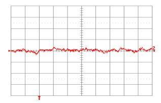
Fig. 12: Input reflected ripple current, is (10 mA/div), measured through 10 µH at the source at full rated load current and Vin = 48 V. Refer to Fig. 11 for test setup. Time scale: 1µs/div.
