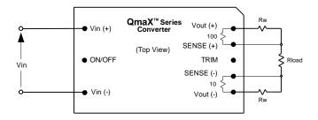
Fig. B: Remote sense circuit configuration.
