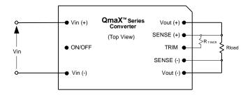
Fig. C: Configuration for increasing output voltage.
