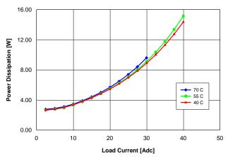
Fig. 6: Power dissipation vs. load current and ambient temperature for converter mounted vertically with Vin = 48 V and air flowing from pin 3 to pin 1 at a rate of 200 LFM (1.0 m/s).
