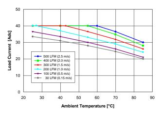
Fig. 1: Available load current vs. ambient air temperature and airflow rates for QM48T40033 converter with B height pins mounted vertically with air flowing from pin 3 to pin 1, MOSFET temperature ≤ 120°C, Vin = 48 V.
