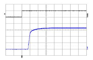
Fig. 7: Turn-on transient at full rated load current (resistive) with no output capacitor at Vin = 48 V, triggered via ON/OFF pin. Top trace: ON/OFF signal (5 V/div.). Bottom trace: output voltage (1 V/div.) Time scale: 2 ms/div.
