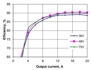
Figure 4. QLS20ZG Efficiency vs. Output Load
