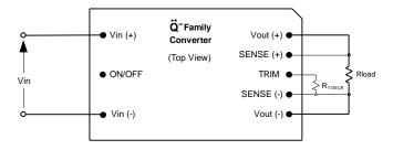
Figure 4. Configuration for decreasing output voltage.
