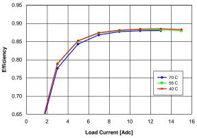
Figure 16. Efficiency vs. load current and ambient temperature for converter mounted horizontally with Vin = 54 V and air flowing from pin 3 to pin 4 at a rate of 200 LFM (1.0 m/s).
