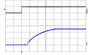
Figure 18. Turn-on transient at full rated load current (resistive) plus 10,000 μF at Vin = 48 V, triggered via ON/OFF pin. Top trace: ON/OFF signal (5 V/div.). Bottom trace: output voltage (2 V/div.). Time scale: 2 ms/div.
