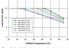
Figure 10. Available load current vs. ambient air temperature and airflow rates for converter mounted vertically with Vin = 54 V, air flowing from pin 3 to pin 1 and maximum FET temperature ≤ 105 °C.
