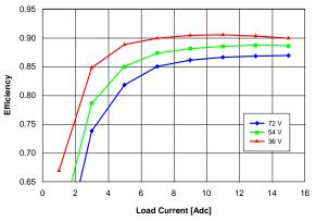
Figure 15. Efficiency vs. load current and input voltage for converter mounted horizontally with air flowing from pin 3 to pin 4 at a rate of 300 LFM (1.5 m/s) and Ta = 25 °C.
