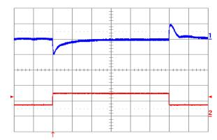
Figure 20. Output voltage response to load current stepchange (3.75 A – 7.5 A – 3.75 A) at Vin = 48 V. Top trace: output voltage (100 mV/div.). Bottom trace: load current (5 A/div). Current slew rate: 5 A/ μs. Co = 450 μF tantalum + 1 μF ceramic. Time scale: 0.2 m
