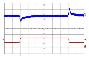
Figure 19. Output voltage response to load current stepchange (3.75 A – 7.5 A – 3.75 A) at Vin = 48 V. Top trace: output voltage (100 mV/div). Bottom trace: load current (5 A/div.). Current slew rate: 0.1 A/ μs. Co = 1 μF ceramic. Time scale: 0.2 ms/div.
