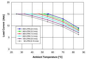
Figure 12. Available load current vs. ambient temperature and airflow rates for converter mounted horizontally with Vin = 54 V, air flowing from pin 3 to pin 4 and maximum FET temperature ≤ 105 °C.
