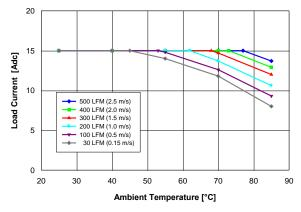
Figure 9. Available load current vs. ambient air temperature and airflow rates for converter mounted vertically with Vin = 54 V, air flowing from pin 3 to pin 1 and maximum FET temperature ≤ 120 °C.
