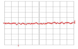
Figure 24. Input reflected ripple current, is (10 mA/div), measured through 10 µH at the source at full rated load current and Vin = 48 V. Refer to Fig. 22 for test setup. Time scale: 1 µs/div.
