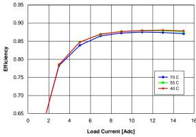
Figure 14. Efficiency vs. load current and ambient temperature for converter mounted vertically with Vin = 54 V and air flowing from pin 3 to pin 1 at a rate of 200 LFM (1.0 m/s).
