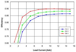
Figure 13. Efficiency vs. load current and input voltage for converter mounted vertically with air flowing from pin 3 to pin 1 at a rate of 300 LFM (1.5 m/s) and Ta = 25 °C.
