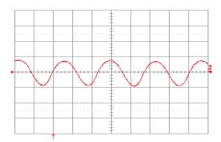
Figure 23. Input reflected ripple current, ic (100 mA/div), measured at input terminals at full rated load current and Vin = 48 V. Refer to Fig. 22 for test setup. Time scale: 1 µs/div.
