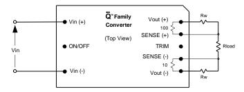
Figure 2. Remote sense circuit configuration.
