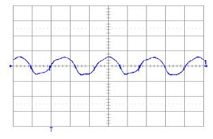
Figure 21. Output voltage ripple (20 mV/div.) at full rated load current into a resistive load with Co = 10 μF tantalum + 1μF ceramic and Vin = 48 V. Time scale: 1 μs/div.
