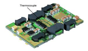
Figure 27. Location of the thermocouple for thermal testing.
