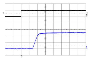
Figure 17. Turn-on transient at full rated load current (resistive) with no out-put capacitor at Vin = 48 V, triggered via ON/OFF pin. Top trace: ON/OFF signal (5 V/div.). Bottom trace: output voltage (2 V/div.) Time scale: 1 ms/div.
