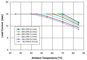
Figure 11. Available load current vs. ambient temperature and airflow rates for converter mounted horizontally with Vin = 54 V, air flowing from pin 3 to pin 4 and maximum FET temperature ≤ 120 °C.
