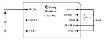
Figure 3. Configuration for increasing output voltage.
