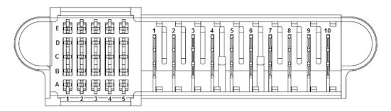
Power Supply Connector: Tyco Electronics P/N 1926736-3 or FCI connector 10133129-002LF or equivalent (NOTE: Column 5 is recessed (short pins))
