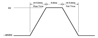
Figure 4. 0 V Line Transient Test
