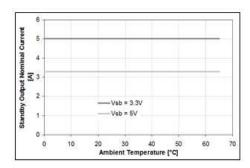
Figure 9. Current Limitation and Temperature Derating on 3.3 / 5  $V_{\rm SB}$
