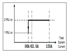
Figure 15. Hot-standby enable/disable current thresholds
