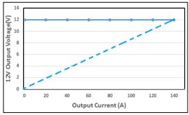
Figure 6. Current Limitation on V1
