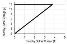
Figure 10. Current Limitation on 12 V<sub>SB</sub>
