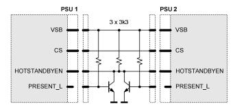
Figure 17. Recommended hot-standby configuration
