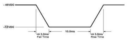
Figure 3. Minus 72 VDC Line Transient Test
