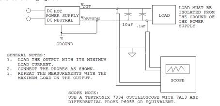
Figure 5. Differential Noise Test Setup
