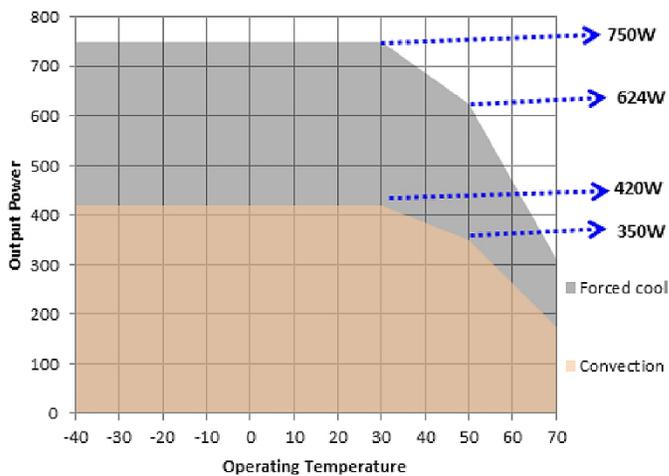
Forced air cooled load: 750 W up to 30°C
