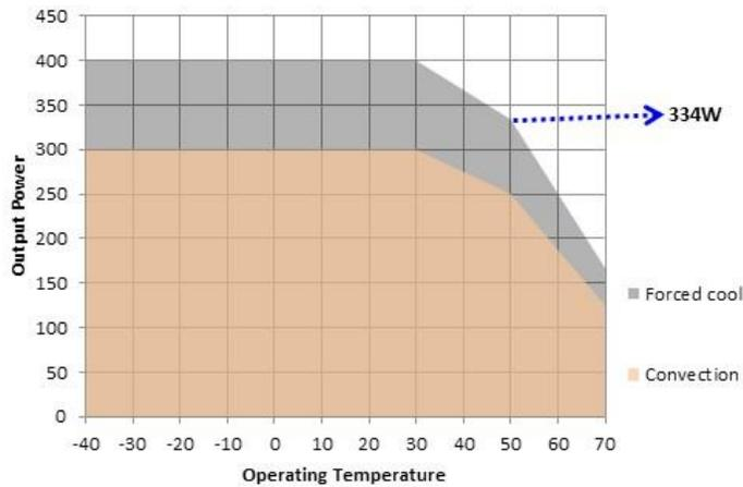
Forced air cooled load: 400 W up to 30°C
