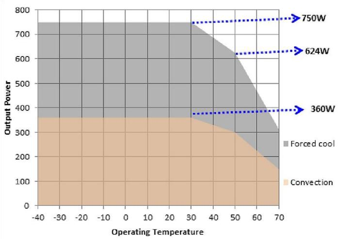
Forced air cooled load: 750 W up to 30°C
