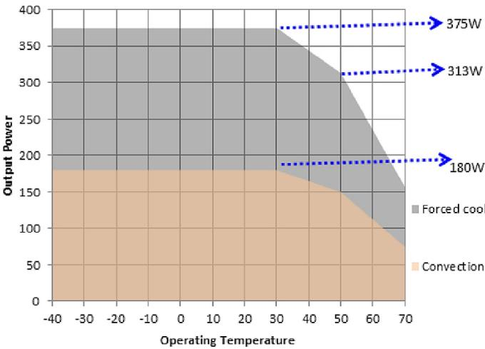
Figure 8. Power Derating Curve 12 V with Plain Cover
