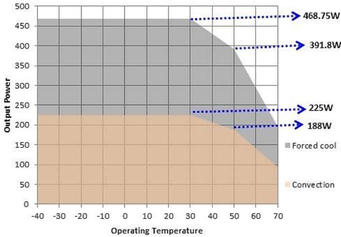
Forced air cooled load: 468.75 W up to 30°C
