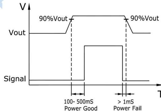
Figure 1. Power Good / Fail Signal Diagram
