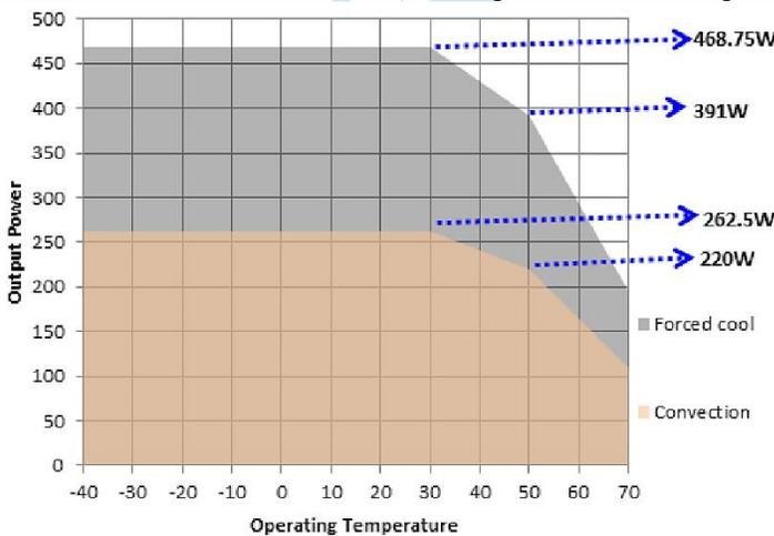
Figure 10. Power Derating Curve 15 V with Slotted Cover
