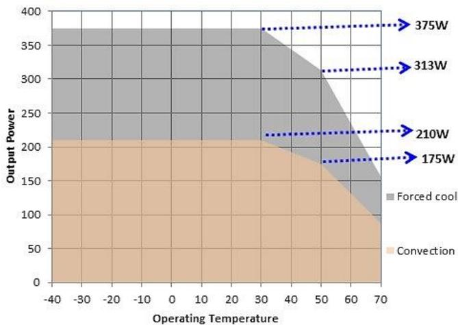
Forced air cooled load: 375 W up to 30°C
