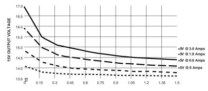
15V OUTPUT CURRENT Figure 3. MAP40-3003G Typical Quasi Regulation Performance For +15V Output
