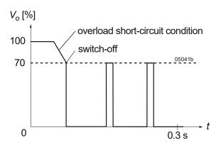
Fig. 6 Overload switch off (hiccup mode), typical values.
