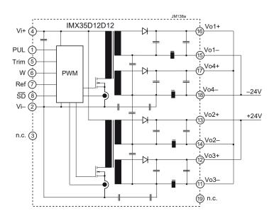
Fig. 7 Generating 24 V with an IMX35D12D12-8
