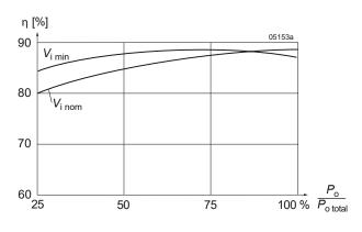
Fig. 11 Efficiency versus input voltage and load. Typical values (20IMX35D12D12-8)
