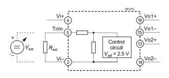
Fig. 13 Output voltage control by means of the Trim input
