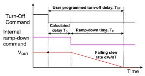
As it can be seen from the figure, the internally calculated delay  $T_{\text{D}}$  is determined by the equation below.
