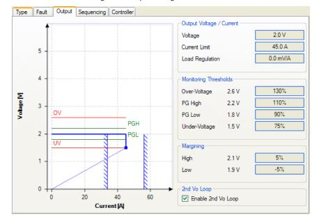
Figure 6. Output Configuration Window
