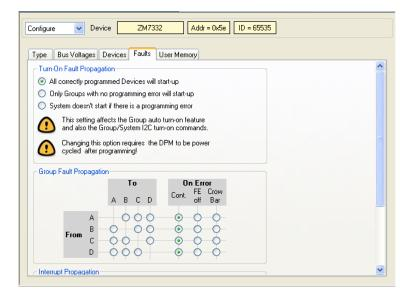
Note that the turn-off type of the fault as it propagates through the DPM will remain unchanged. Propagation options for dPOLs can be read or set in the dPOL PC3 register shown in Figure 30.
