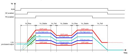
Figure 25. Protections Enable Conditions
