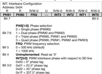
Figure 37. Interleave Configuration Register INT
