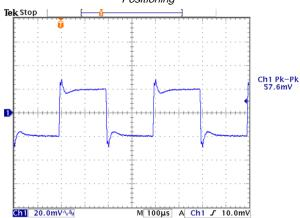
As the Load Regulation parameter is increased, step offsets in output voltage begin to appear, as shown in Figure 9.
