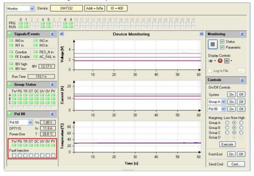
Figure 47. Fault Injection Controls In Monitor Window
