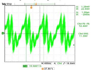
Figure 39. Input Voltage Noise with Interleave
