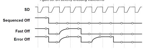
Figure 35. OK Severity Encoding Waveforms
