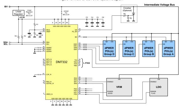
Figure 49. Multi-dPOL Power System Diagram
