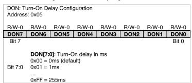
Figure 12. Turn-On Delay Register DON
