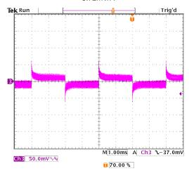
As noted earlier, increasing the Load Regulation parameter provides load dependant dynamic load positioning. This shows up in Figure 44.
