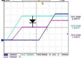
Figure 20 was captured with an actual system where a diode was added to pre-bias a 1.5V bus from a 1.85V bus in order to simulate the effect of current leakage through protection circuits of unpowered logic connected to powered logic outputs (a common source of pre-bias in power systems).
