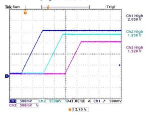
V1 at 1.0V/ms, V2 at 0.5V/ms, V3 at0.2V/ms. Vin=12V
