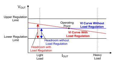
Figure 8. Concept of Optimal Voltage Positioning
