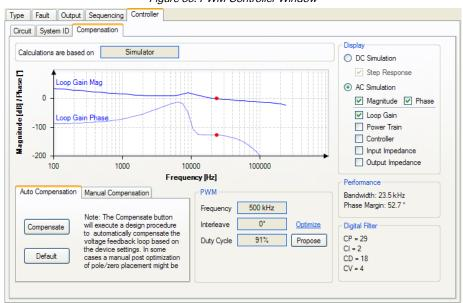
Figure 36. PWM Controller Window
