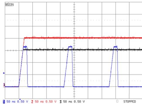
Figure 35 shows a scope capture an actual system when undervoltage error detection is set to not propagate.
