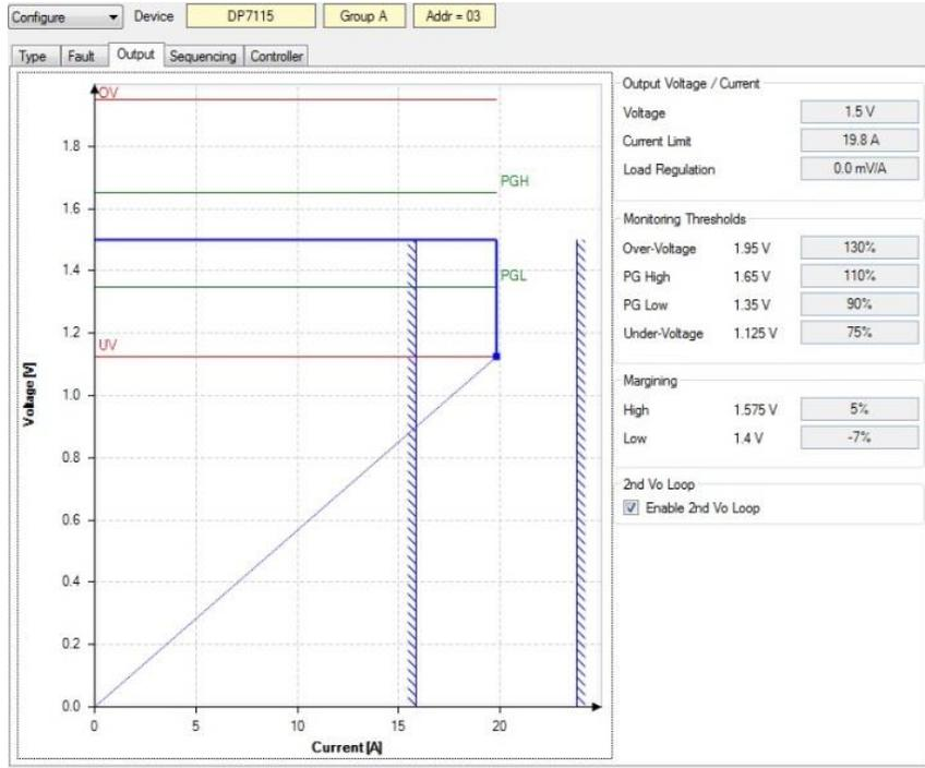
Note that the GUI shows the effect of setting PG, OV and UV limits as both values and graphical limit bars. Vertical hashed lines are error bars for the Overcurrent (OC) limit.
