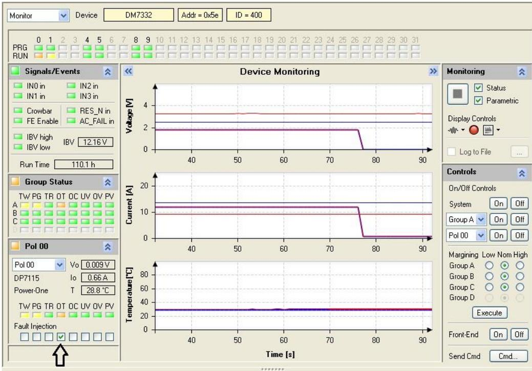
In Figure 51 we see the effects of injecting an Overtemp (OT) fault. Note that dPOL-0 shows an OT fault. DPOL-0 and -1 are in the same Group and fault propagation for the dPOL is to propagate to the group. dPOL -4 and above are in Groups B and C. Propagation is not enabled from Group A to B.
