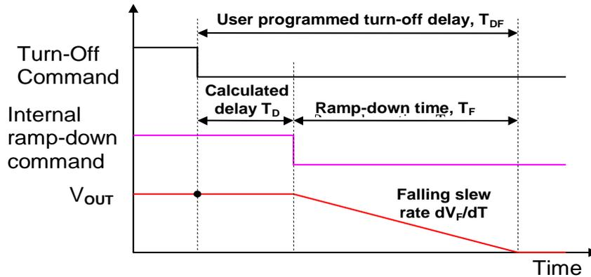
As it can be seen from Figure 16, the internally calculated delay T<sub>D</sub> is determined by the equation below.
