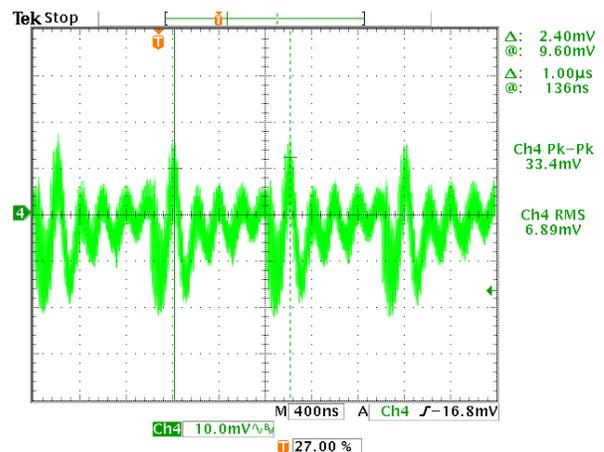
Figure 42 shows the input voltage noise of the three-output system with programmed interleave. Instead of all three dPOLs switching at the same time as in the previous example, the switching cycle of dPOLs V1, V2, and V3 start at
