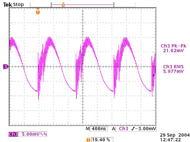
Figure 42. Output Voltage Noise, Full Load, 180° Interleave
