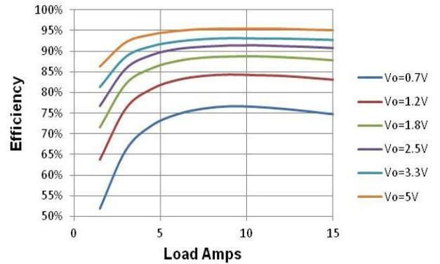
Figure 9 Efficiency vs Vout, Fsw=500KHz
