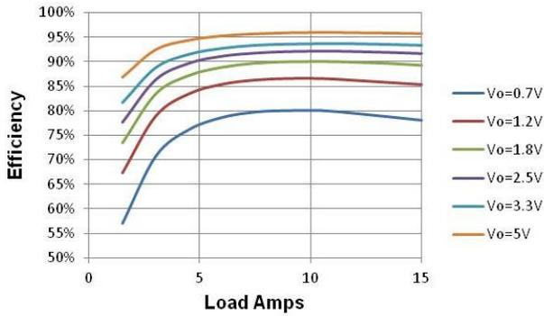
Figure 8 Efficiency vs Load, Vin=8V, Fsw=1MHz
