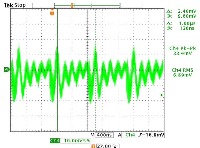
Figure 46 shows the input voltage noise of the three-output system with programmed interleave. Instead of all three dPOLs switching at the same time as in the previous example, the dPOLs V1, V2, and V3 switch at 67.5°, 180°, and 303.75°, respectively. Noise is spread evenly across the switching cycle resulting in more than 1.5 times reduction. To achieve similar noise reduction without the interleave will require the addition of an external LC filter.
