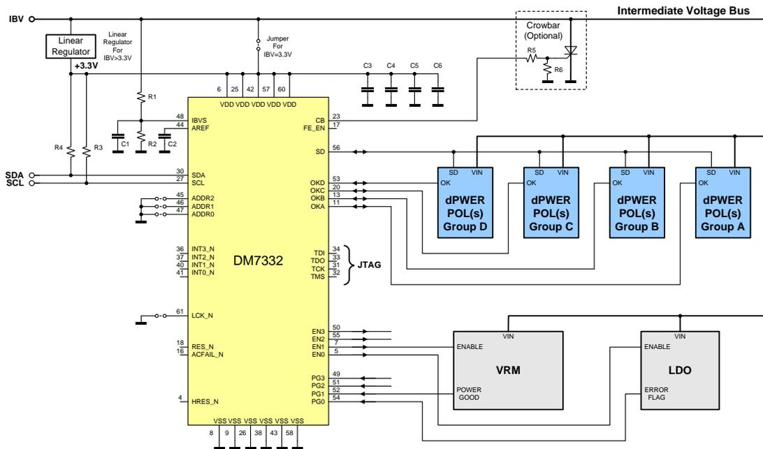
Shown in Figure 57 is a schematic of a typical application using at least one DP7115G point-of-load converter (dPOL). The system includes a DM7300 series Digital Power Manager (DPM), a DP7115G dPOL. Although only one dPOL is shown, other, additional d-pwer® series dPOLs (Note SD and OK dashed lines "TO OTHER POLS") may be connected.
