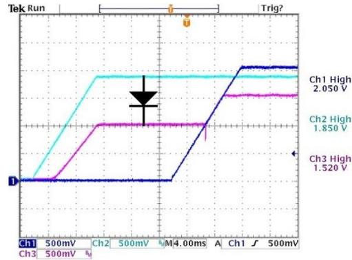
Figure 27 was captured with an actual system where a diode was added to pre-bias a 1.5V bus from a 1.85V bus in order to simulate the effect of current leakage through protection circuits of unpowered logic connected to powered logic outputs (a common source of pre-bias in power systems).
