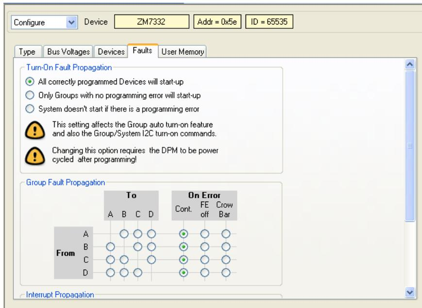
Note that the turn-off type of the fault as it propagates through the DPM will remain unchanged. Propagation options for dPOLs can be read or set in the dPOL PC3 register shown in Figure 37.
