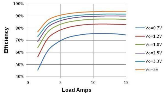
Figure 7 Efficiency vs Load, Vin=8V, Fsw=500KHz
