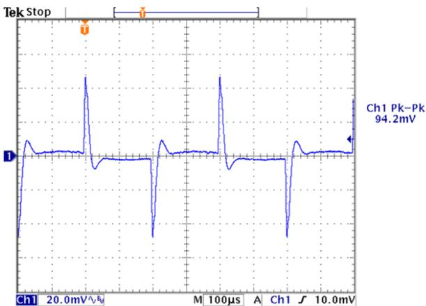
Figure 17 Transient response with non-zero Regulation.
