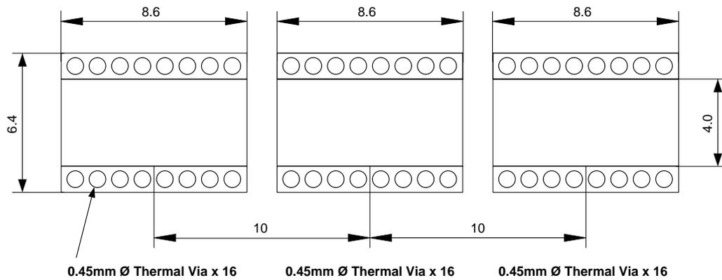
0.45mm Ø Thermal Via x 16      0.45mm Ø Thermal Via x 16      0.45mm Ø Thermal Via x 16
