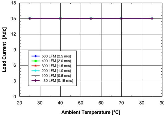
Figure 2. Available output current vs. ambient air temperature and airflow rates for converter DP7115G mounted horizontally with air flowing from input to output, MOSFET temperature  $\leq 120^\circ\text{C}$ ,  $V_{in} = 8\text{ V}$ ,  $V_{out} = 5\text{ V}$ , and  $F_{sw} = 1\text{MHz}$
