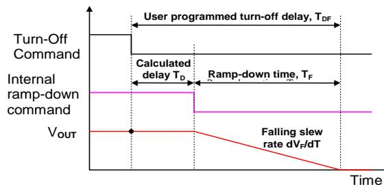
As it can be seen from the figure, the internally calculated delay  $T_D$  is determined by the equation below.
