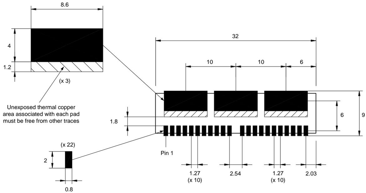
Figure 61. Recommended PCB Power Tab (Pins 23 - 25) Layout for Multilayer PCBs
