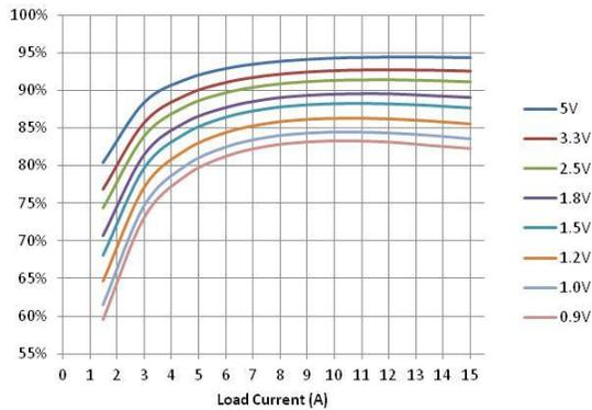
Figure 6. Efficiency vs. Load.  $V_{in} = 12\text{V}$ ,  $F_{sw} = 1\text{MHz}$
