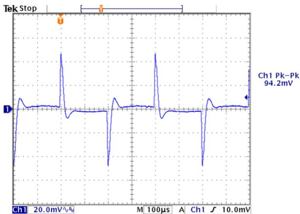
Figure 17 Transient response with non-zero Regulation.
