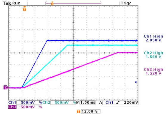
Figure 25. Sequenced Turn-On. Rising Slew Rate is Programmed at 1V/ms. V2 Delay is 2ms, V3 delay is 4ms.
