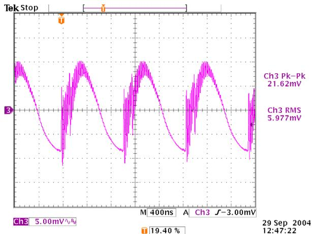
Figure 48. Output Voltage Noise, Full Load, 180° Interleave
