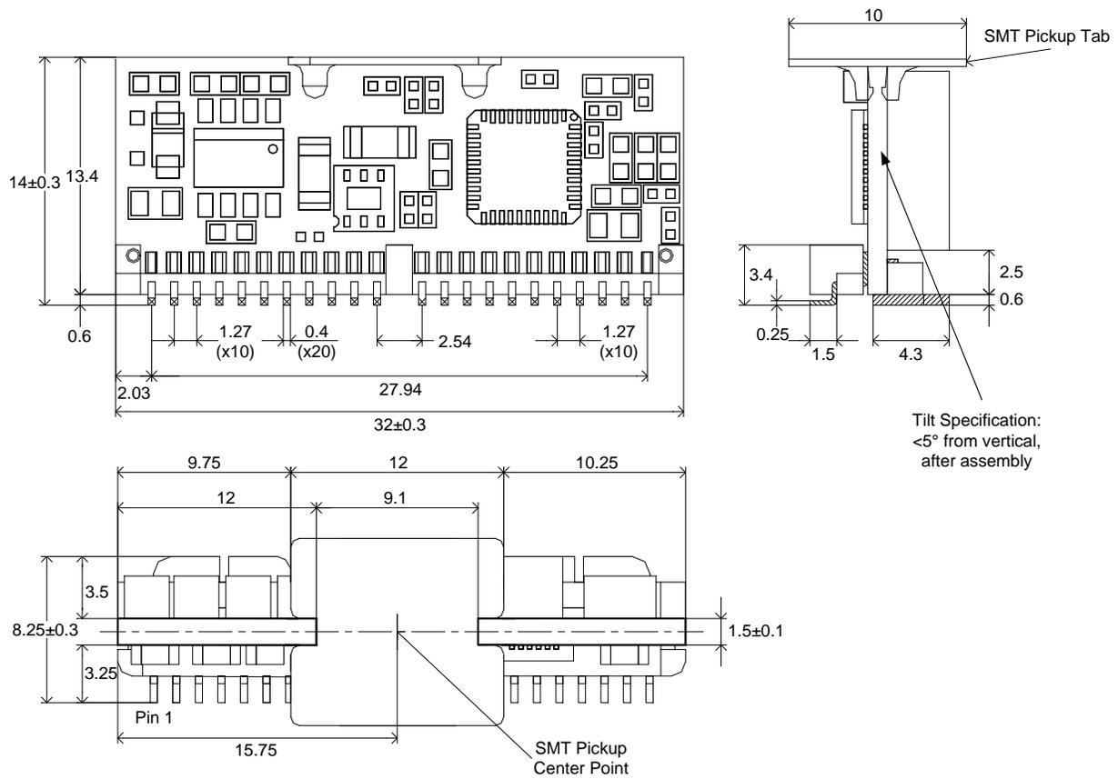
Figure 59. Pinout Diagram (Bottom View)
