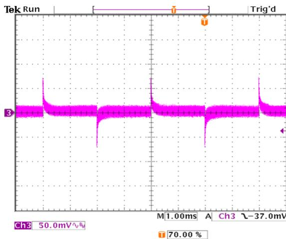
Figure 51. Transient Response with Regulation set to 3.72 mV/A.
