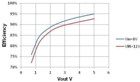
Figure 3. Efficiency vs. Output Voltage,  $I_{out}=15A$ ,  $F_{sw}=500kHz$
