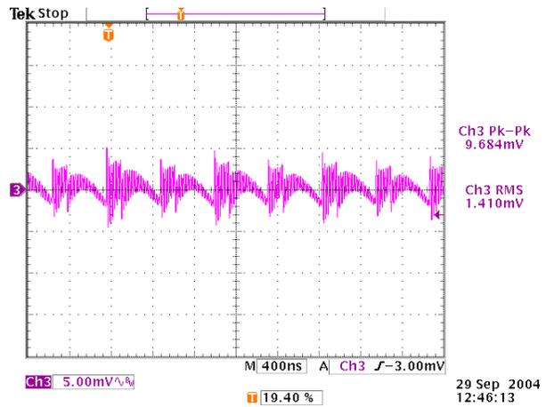
Figure 45. Output Voltage Noise, Full Load, 180° Interleave
