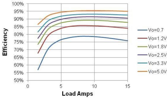
Figure 1. Efficiency vs. Load.  $V_{in}=8V$ ,  $F_{sw}=500kHz$
