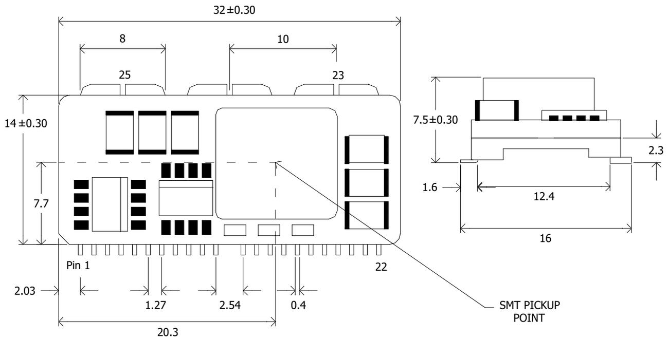
Figure 52. Mechanical Drawing
