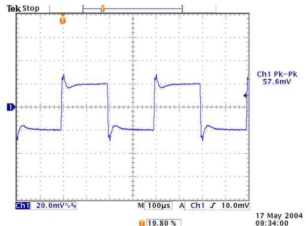
Figure 15. Transient Response with Optimal Voltage Positioning
