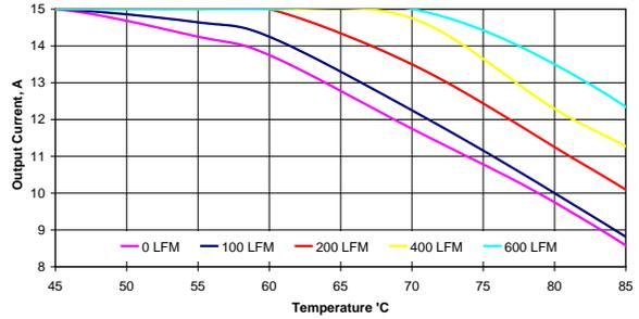
Figure 10. Thermal Derating Curves. Vin=13.2V, Vout=5.0V, Fsw=1MHz
