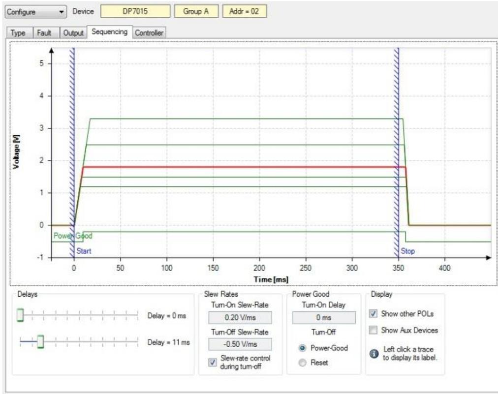
Figure 16. Sequencing/Tracking Window
