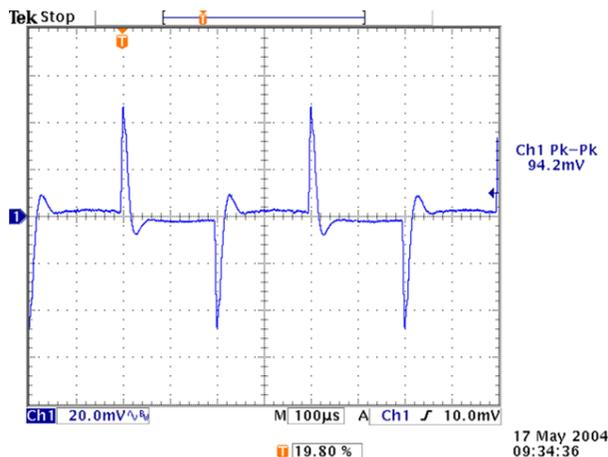
Figure 14. Transient Response without Optimal Voltage Positioning
