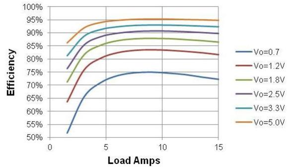
Figure 4. Efficiency vs. Load.  $V_{in}=8V$ ,  $F_{sw}=1MHz$
