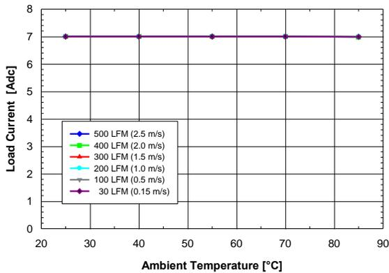
Figure 1. Available output current vs. ambient air temperature and airflow rates for converter DP7007G mounted horizontally with air flowing from input to output, MOSFET temperature  $\leq 120^{\circ}\text{C}$ ,  $V_{in} = 12\text{ V}$ ,  $V_{out} = 5\text{ V}$ , and  $F_{sw} = 500\text{ kHz}$
