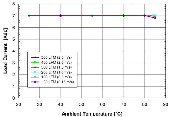
Figure 2. Available output current vs. ambient air temperature and airflow rates for converter DP7007G mounted horizontally with air flowing from input to output, MOSFET temperature  $\leq 120^{\circ}\text{C}$ ,  $V_{in} = 12\text{ V}$ ,  $V_{out} = 5\text{ V}$ , and  $F_{sw} = 1\text{ MHz}$
