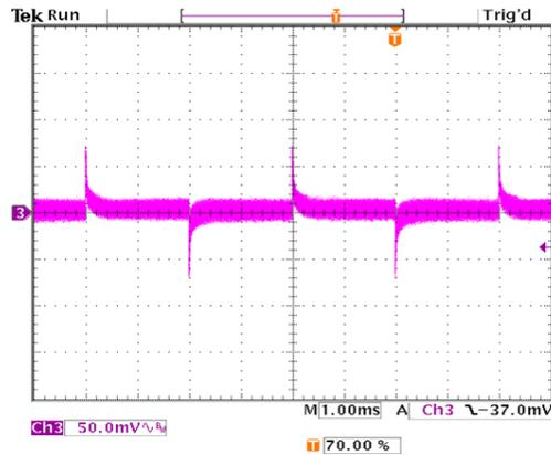
Figure 43. Transient Response with Regulation set to 0.0 mV/A.
