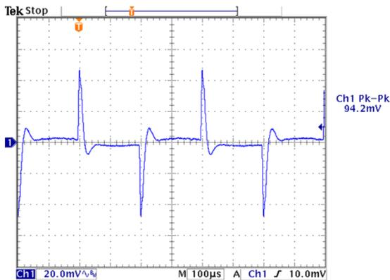
Figure 9 Transient Response with Regulation set to 0 mV/A
