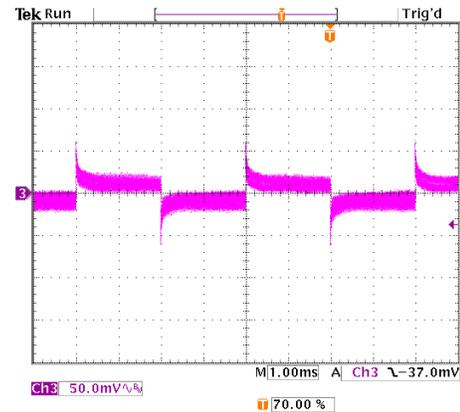
Figure 44. Transient Response with Regulation set to 3.72mV/A
