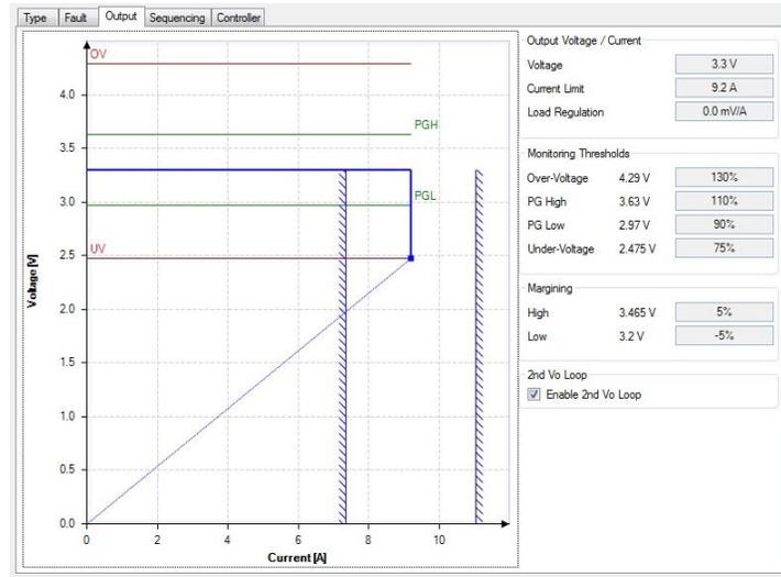
Figure 6. Output Configuration Window
