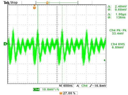
Figure 39. Input Voltage Noise with Interleave
