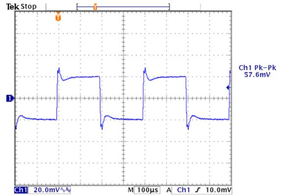
Figure 10 Transient response with Regulation set to 2.23mV/A.
