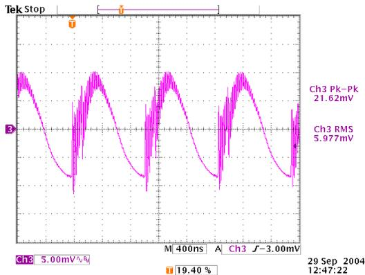
Figure 40. Output Voltage Noise, Full Load, No Interleave
