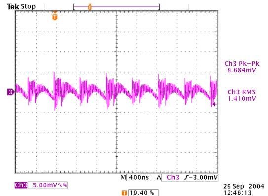
Figure 41. Output Voltage Noise, Full Load, 180° Interleave
