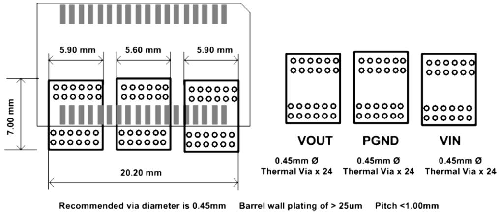
Figure 55. Recommended PCB Layout for Multilayer PCBs
