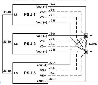
Figure 7. Current Sharing Block Diagram
