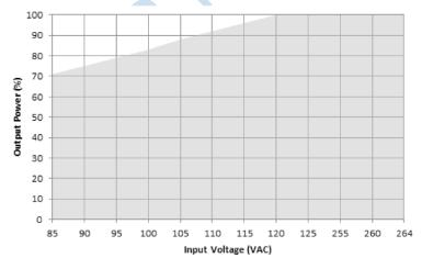
Figure 2. Power Derating w.r.t Input
