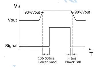
Figure 1. Power Good / Fail Signal Diagram
