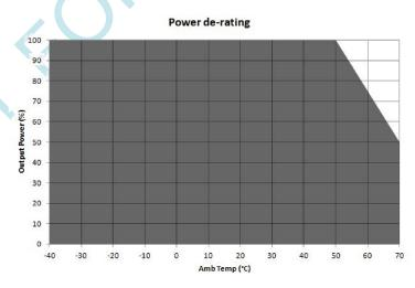
Figure 1. Derating Curve for all Outputs
