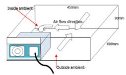
The 12V main output is de-rated at different ambient condition and input condition as below table:
