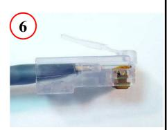
Place wires and management bar into plug housing
