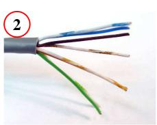
Untwist the pairs and Straighten the Wires
