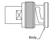
4) Insert the cable and parts into the connector body. Tighten the clamp nut using appropriate wrenches.
