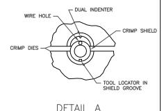
A. PUSH ASSY INTO BODY ASSY UNTIL BOTTOMED, HOLD ASSY FIRMLY BOTTOMED UNTIL FULLY HEX CRIMPED USING MILITARY CRIMP TOOL M22520/5-01 WITH TEI DIE SET CD5-120 OR DANIELS DIE SET Y789(F) CLOSURE "A"
