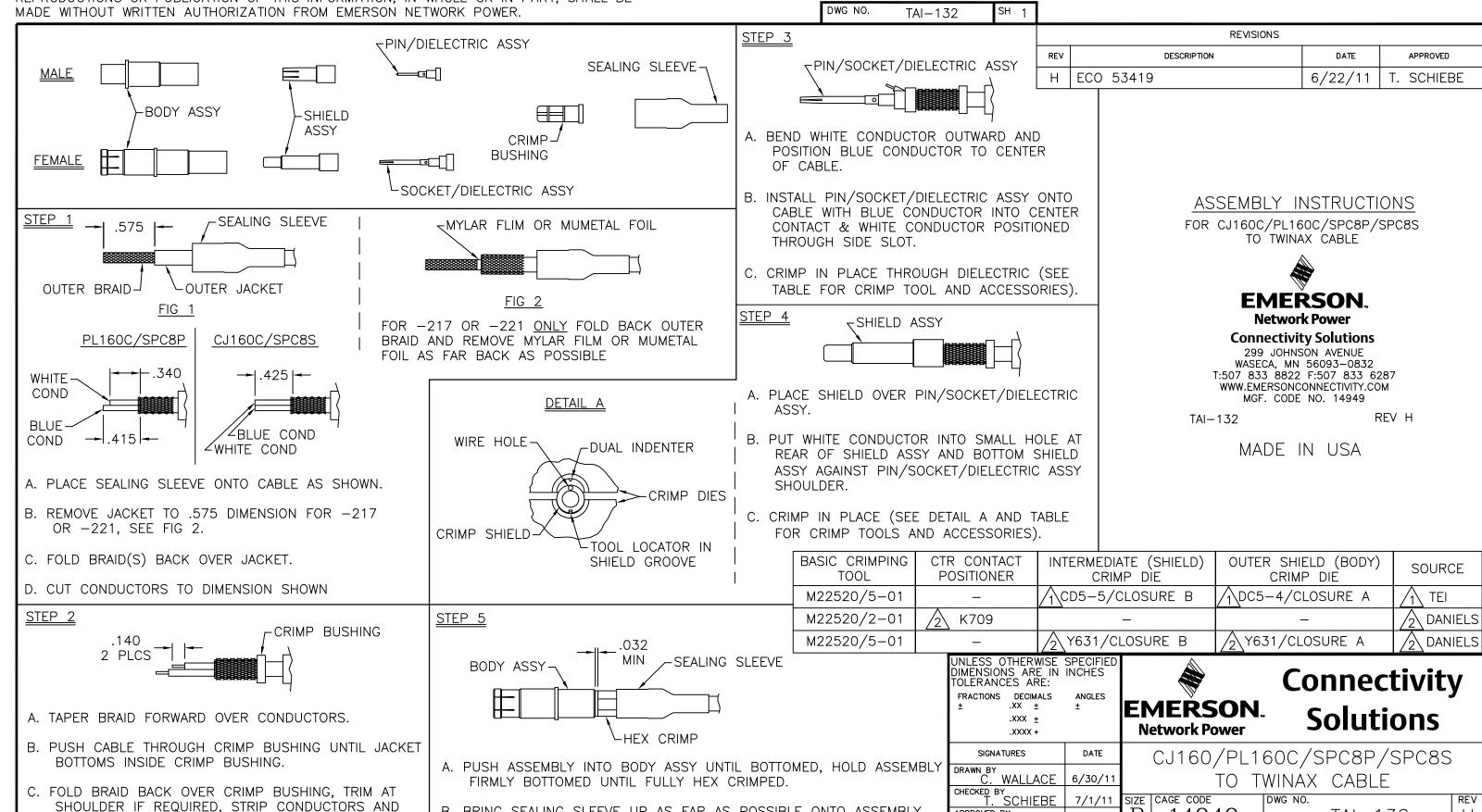
B. BRING SEALING SLEEVE UP AS FAR AS POSSIBLE ONTO ASSEMBLY
