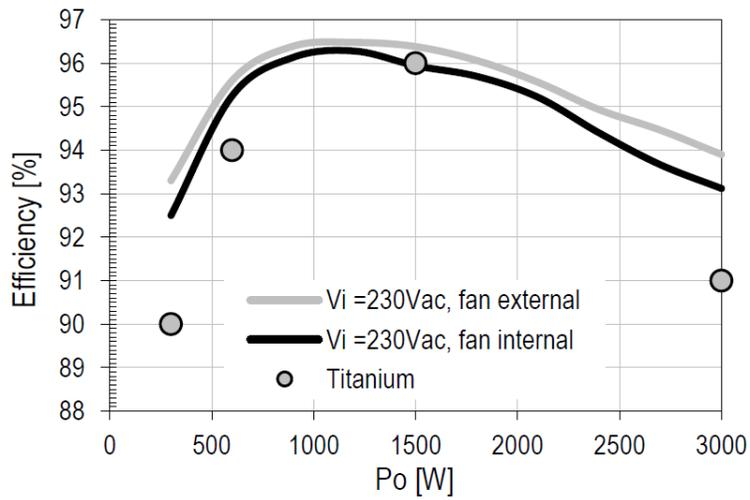
Figure 2. Titanium Efficiency vs. Output Power
