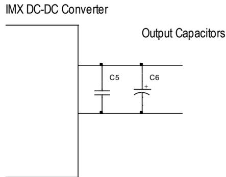
Figure 2 - Capacitance on the output of converter
