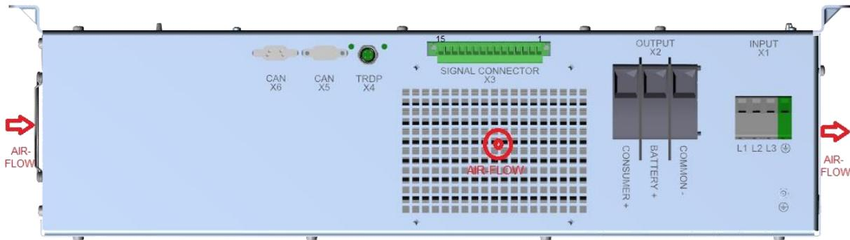
Figure 2. Connector Positions
