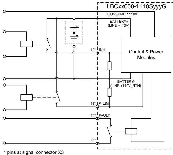
Figure 5. Static signals, connection example
