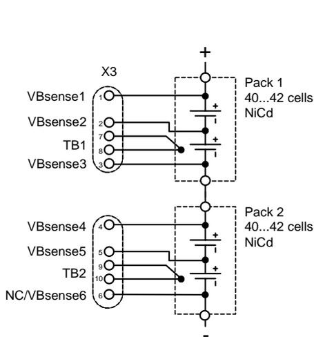
Figure 4. Battery pack sensing
