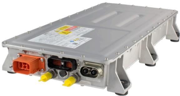
The Bel Power Solutions BCL25-700-8 is a 22/25 kW bi-directional liquid-cooled on-board inverter battery charger with export functionalities for hybrid (HEV) or full electric (EV) vehicles.
