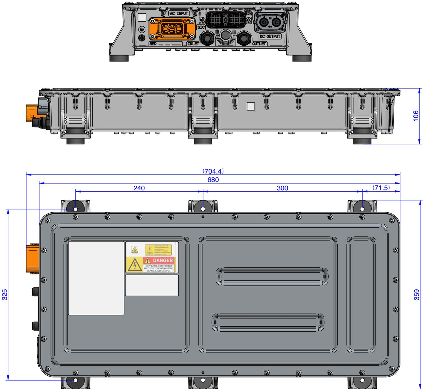
Figure 1. Mechanical Dimensions
