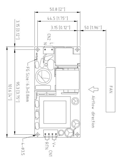
Note: 5. Ensure adequate clearance for components.
