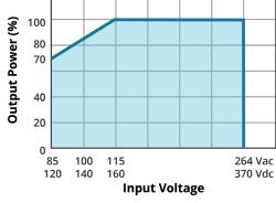
Note: With an AC input voltage between 85 ~ 115 and a DC input between 120 ~ 160 Vdc the output power must be derated as per the temperature derating curve.
