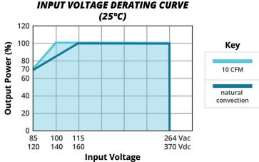
Note: With an AC input voltage between 85 ~ 115 and a DC input between 120 ~ 160 Vdc the output power must be derated as per the temperature derating curve.
