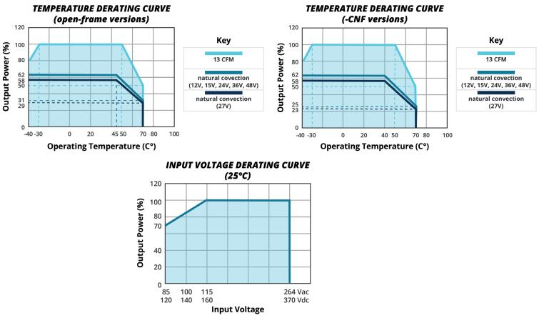
Note: With an AC input voltage between 85 ~ 115 and a DC input between 120 ~ 160 Vdc the output power must be derated as per the temperature derating curve.
