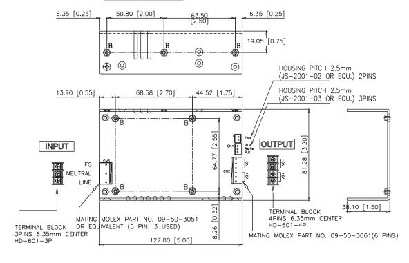
B:MOUNTING HOLE 7 PLACES SACLE4:1 MAXIMUM PENETRATION LENGTH=2.1MM
