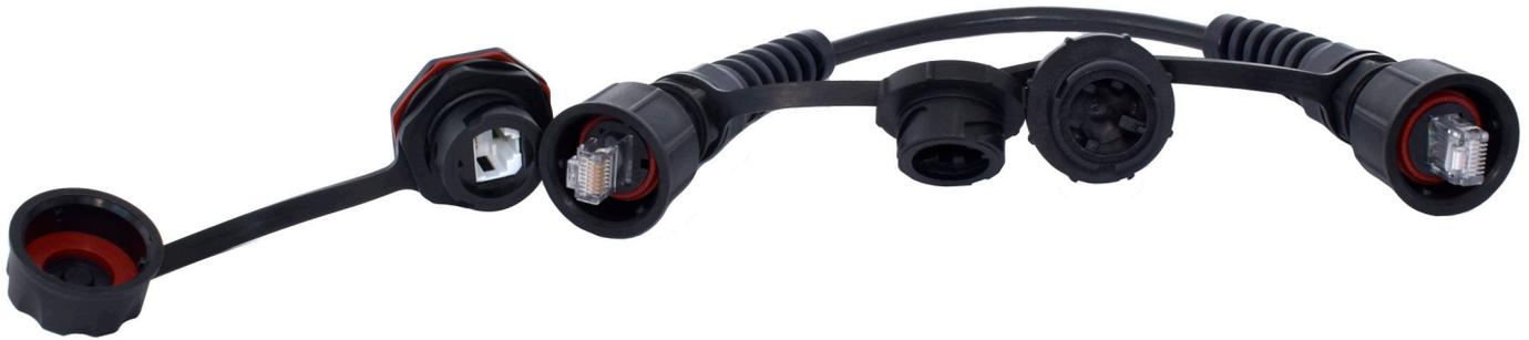
Based on Stewart Connector's RJ45 modular plugs and jack coupled with a sealed IP67 shell design, the SealJack assembly and jack combination is also available for CAT5E and CAT6 applications and in shielded and unshielded configurations. Also RoHS compliant and supporting POE+, as well as 10/100Base-T, 1G Base-T, 2.5G Base-T, and 5G Base-T Ethernet.
