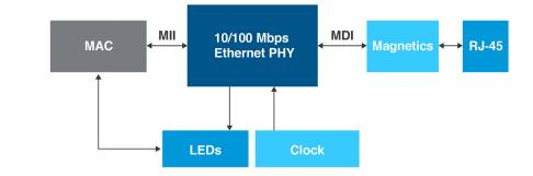
Figure 1: Ethernet PHY connection with MAC and physical medium.
