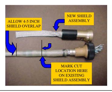
4.4 Put the new backshell, with its attached lightning shield, next to the wires and contacts of the existing backshell/shield assembly. Make a mark on the existing shield to keep five more inches of shield overlap when the retrofit assembly is installed.
