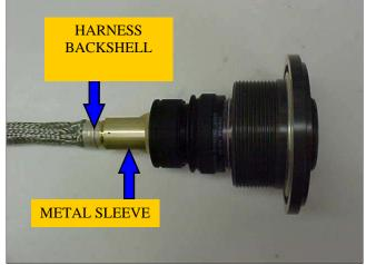
4.0 Cut and remove the lock wire located between the black accessory nut on the CN1156-2 or CN1156-4 plug connector and the backshell. Then loosen (counterclockwise) the black accessory nut that holds the backshell to the plug connector. Then remove the black accessory nut and slide it down the harness.
