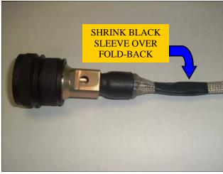
**4.18** Fold back the 1 ½ inch long end section of the tan Expando sleeving over the lacing tape. Slide the 2 inch long black sleeve over the section that is folded back to fully cover the area, then heat shrink the black sleeve into position.
