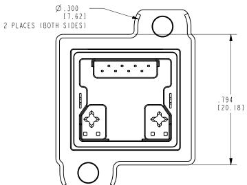
CONNECTOR MATERIALS: HOUSING/INSERT: THERMOPLASTIC UL94 V-0 SHIELD: ZINC DIE-CAST ALLOY SHIELD PLATING: TIN OVER COPPER CONTACTS: COPPER ALLOY CONTACT PLATING: SEE TABLE BELOW GASKET: SILICONE RUBBER SILICONE SEALING COMPOUND IN REAR OF JACK
