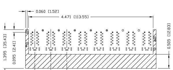
THE SHADED AREA ON THE CUSTOMER BOARD ARE RECOMMENDED TO BE CLEAR OFF ANY VIA HOLE OR COMPONENT PAD.
