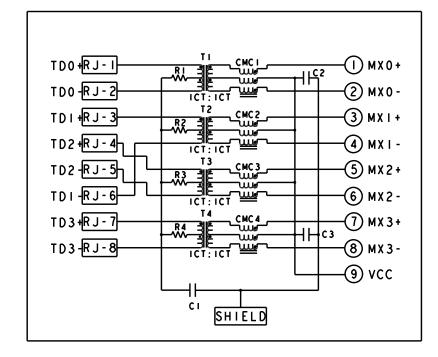
C1 = 1000PF, 2KV, DECOUPLING CAPACITOR C2 - C3 = 10NF, 50V CAPACITORS R1-R4 = 75 OHMS, 1/16 W, RESISTORS
