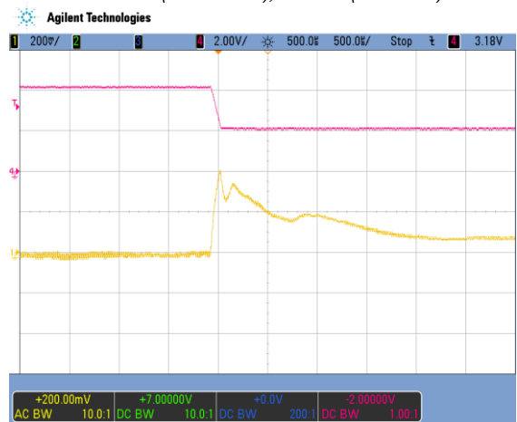
Figure 18. Load transient V1, 244 to 122 A (500 \mu s/div)
