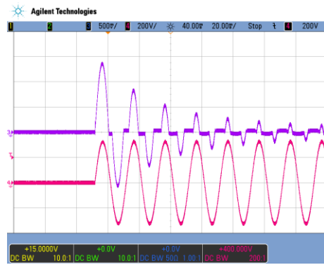
Figure 5 - Inrush current, V_{in} = 230 \text{ Vac} , 0^\circ phase angle CH4: V_{in} (200 V/div), CH3: I_{in} (10 A/div)
